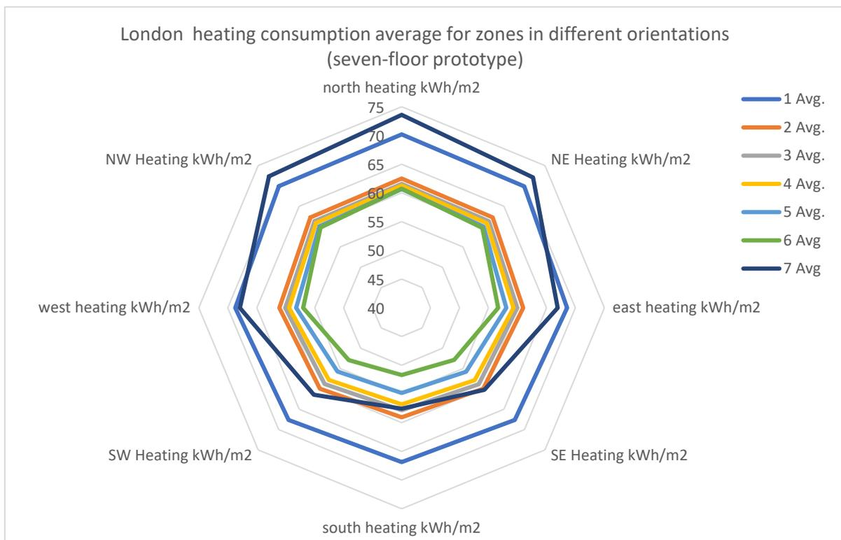
Figure 4-38 Seven-floor prototype heating consumption results average per orientation for London, UK
