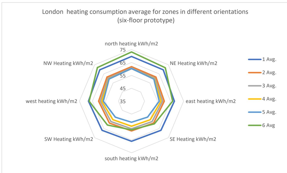
Figure 4-35 Six-floor prototype heating consumption results average per orientation for London, UK
