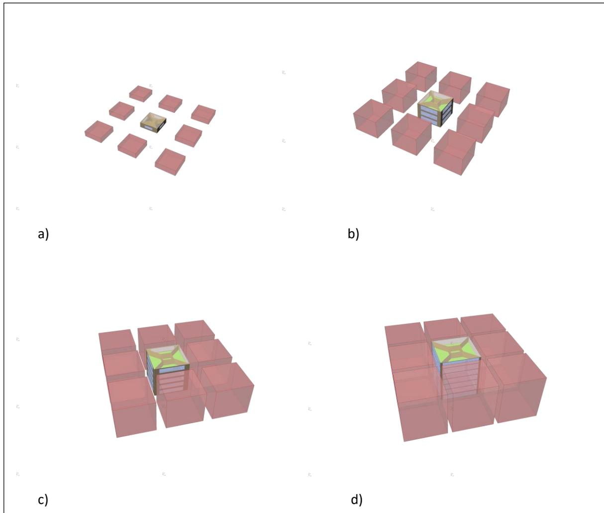
Figure 4-5 Geometrical variables examples a) one-floor height, 20% WWR, 50% built area ratio and zero degrees rotation. b) Three-floor height, 50% WWR, 70% built area ratio and zero degrees rotation. c) Five-floor height, 50% WWR, 80% built area ratio and 45 degrees
