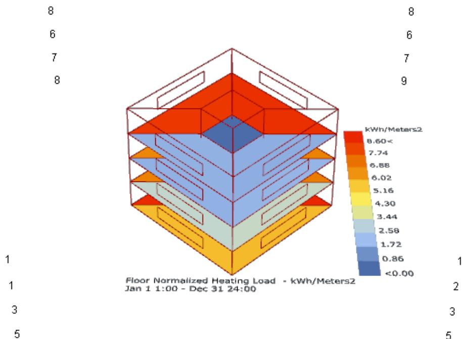
Figure 4-7 Heating consumption in kWh/m2 for each zone for the mentioned case
