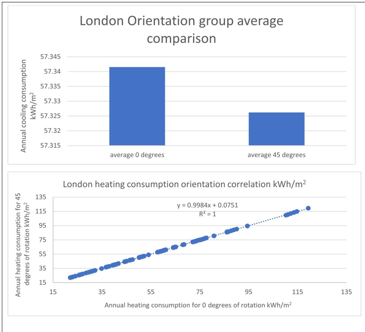
Figure 4-16 Orientation variations' heating consumption average comparison in kWh/m<sup>2</sup>, orientation variations' bound correlated in kWh/m<sup>2</sup> for London, UK
