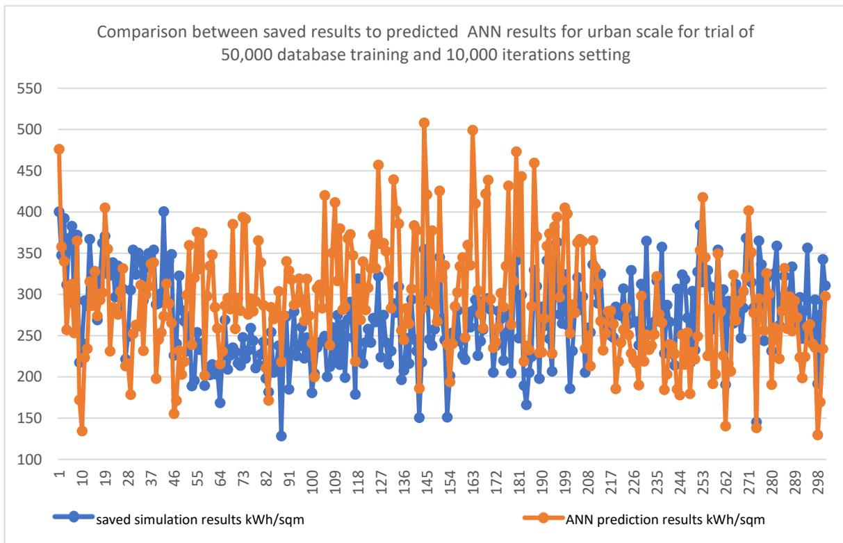
Figure 7-6 Comparison between simulation and prediction results for 300 configurations with ANN trained on 50,000 entries and 10,000 iterations setting.
