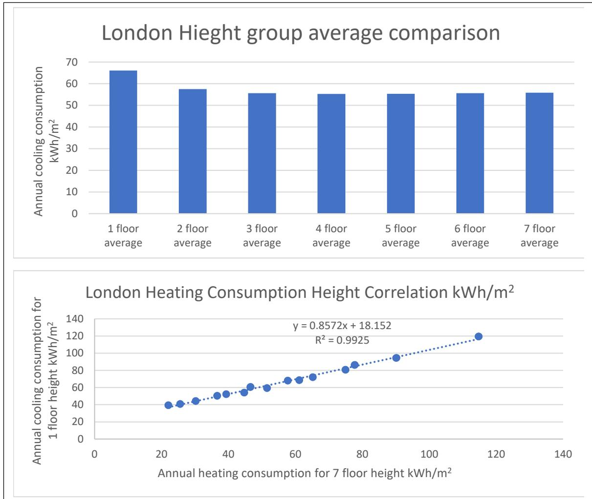
Figure 4-13 Different height groups’ relative importance for heating, cooling and lighting (with dimming) energy consumption for London, UK
