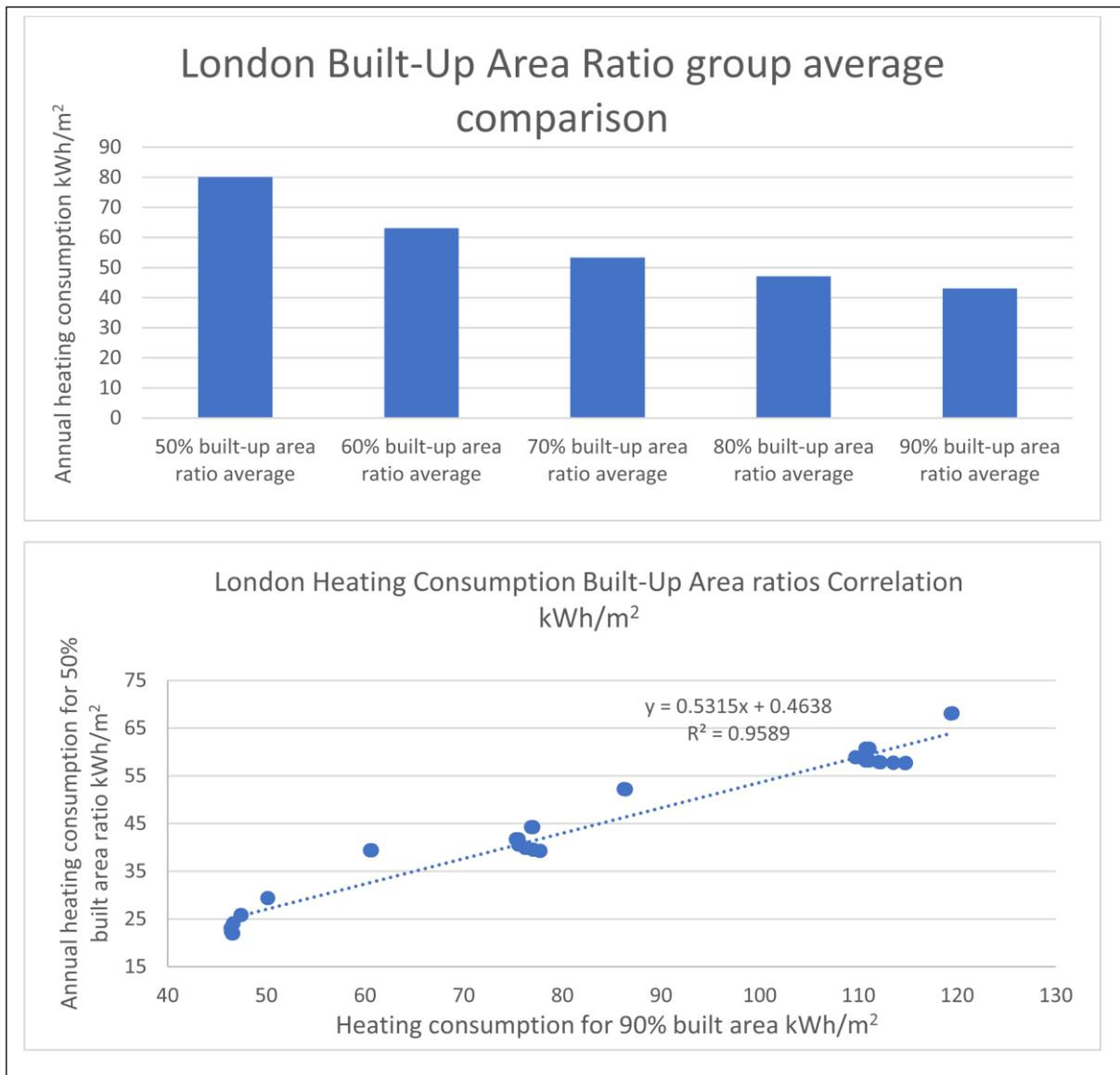
Figure 4-14 Built-up area ratio variations’ heating consumption average comparison in kWh/m<sup>2</sup>, built-up area ratio variations’ bound correlated in kWh/m<sup>2</sup> for London, UK
