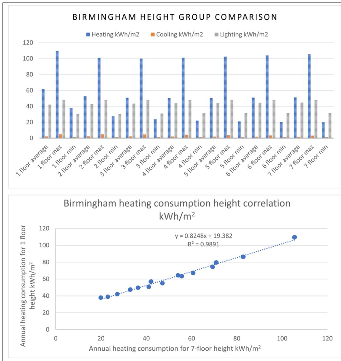
Figure of Different height groups' relative importance for heating, cooling and lighting (with dimming) energy consumption for Birmingham, UK
