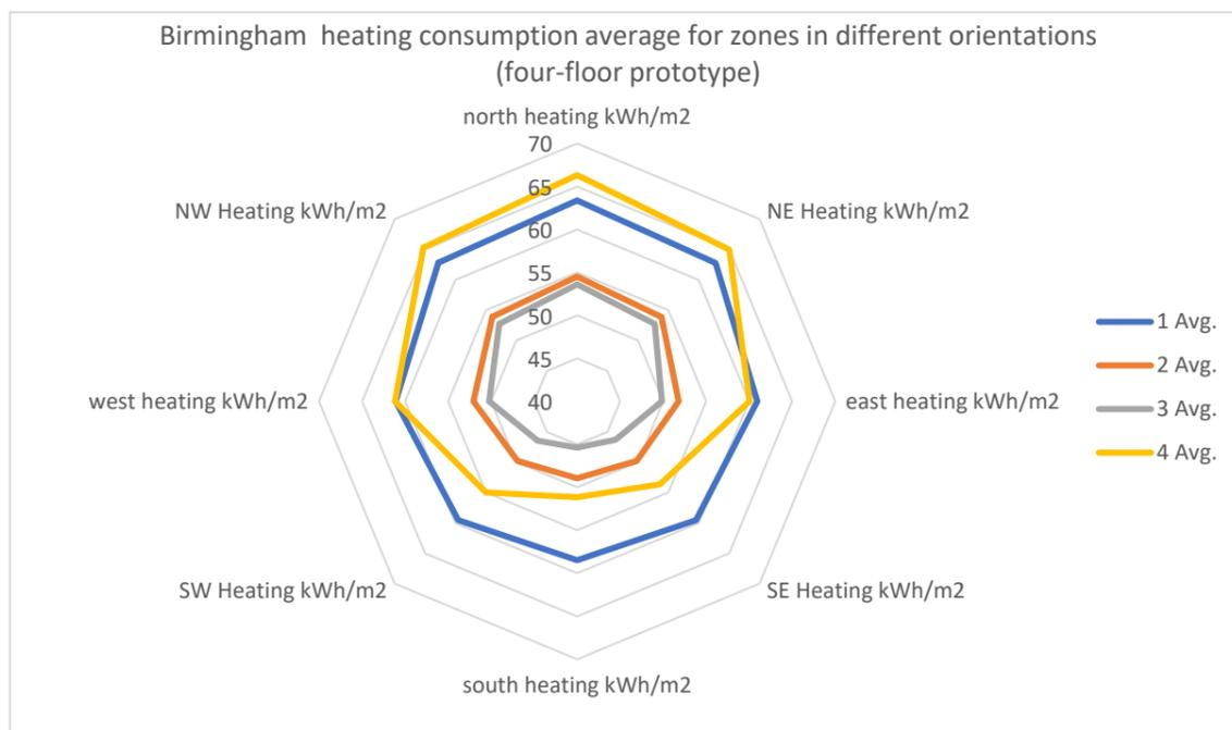
Figure of Four-floor prototype heating consumption results average per orientation for Birmingham, UK
