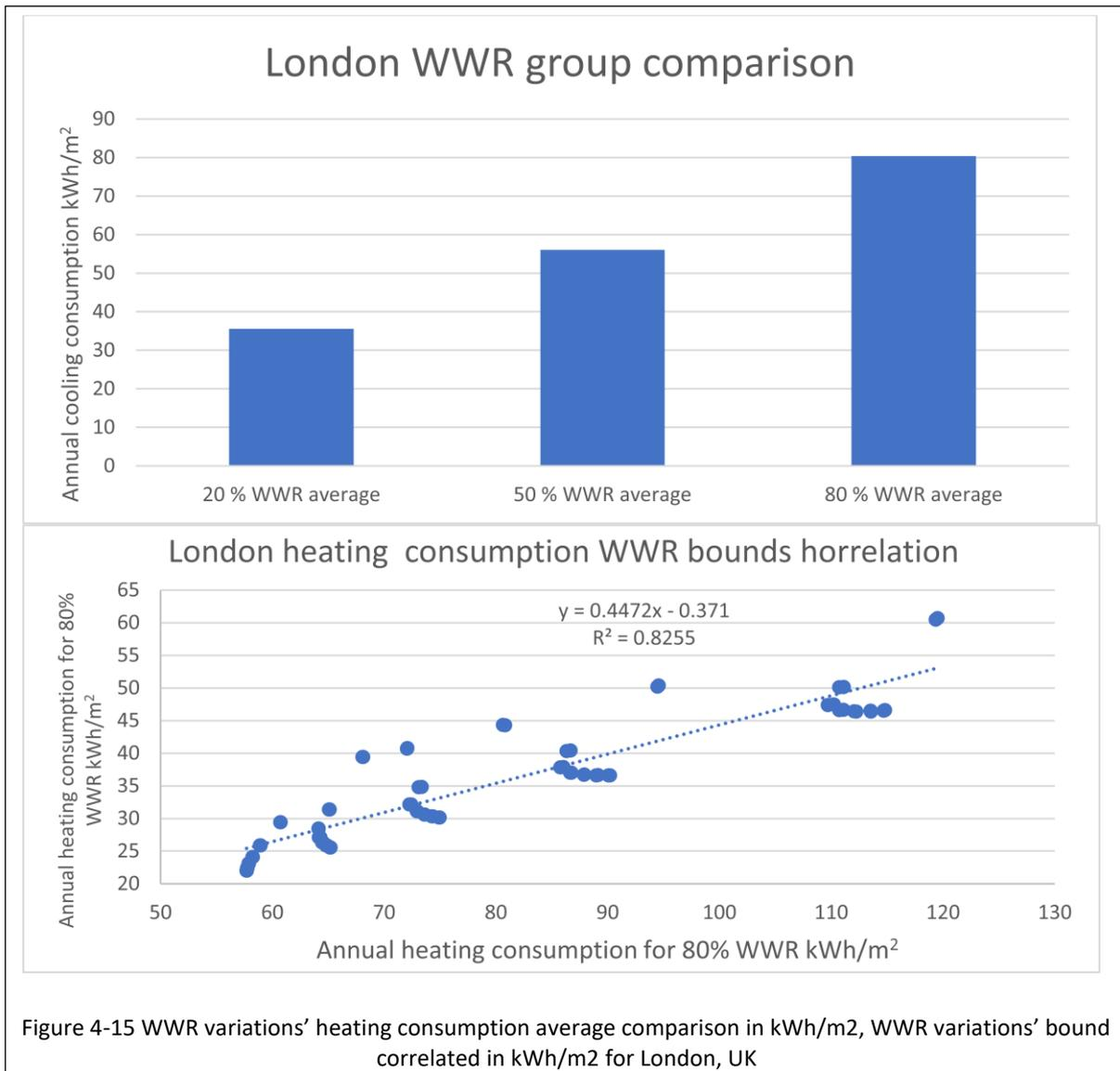
Figure 4-15 WWR variations' heating consumption average comparison in kWh/m2, WWR variations' bound correlated in kWh/m2 for London, UK
