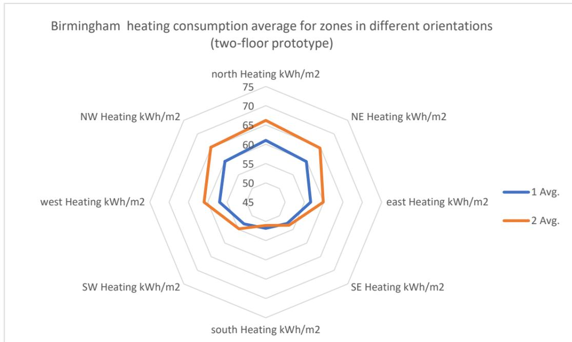
Figure of Two-floor prototype heating consumption results average per orientation for Birmingham, UK
