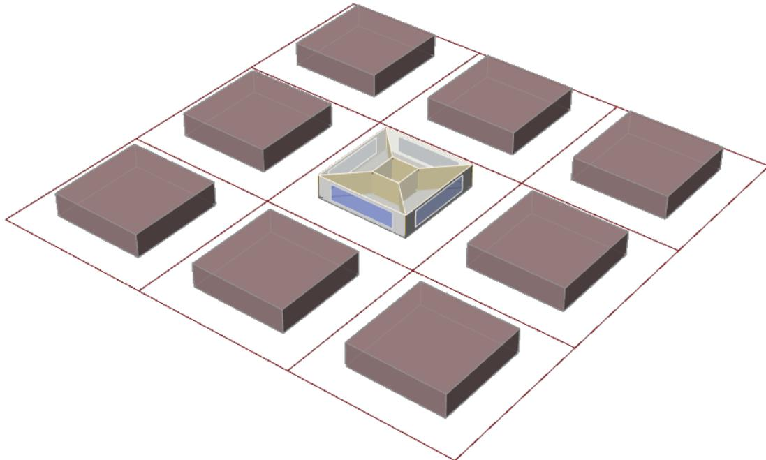
Figure 4-18 One-floor prototype with 50% WWR and 60% built area ratio and no rotation
