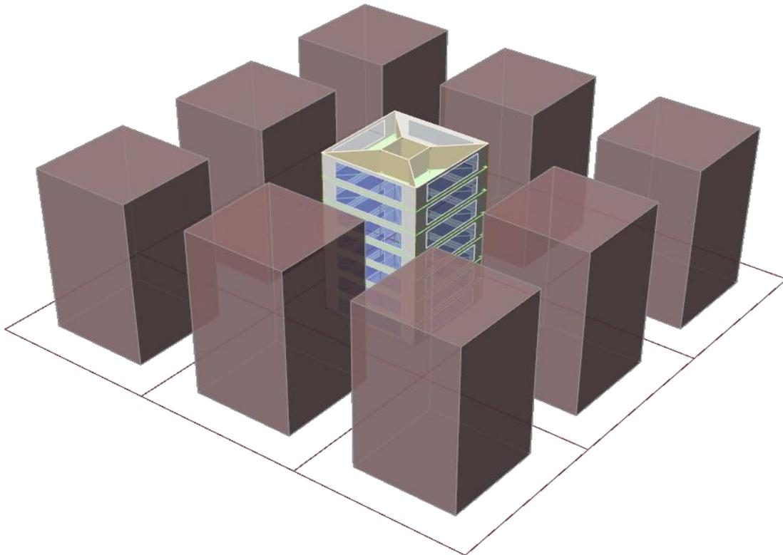
Figure 4-36 Seven-floor prototype with 50% WWR and 60% built area ratio and no rotation
