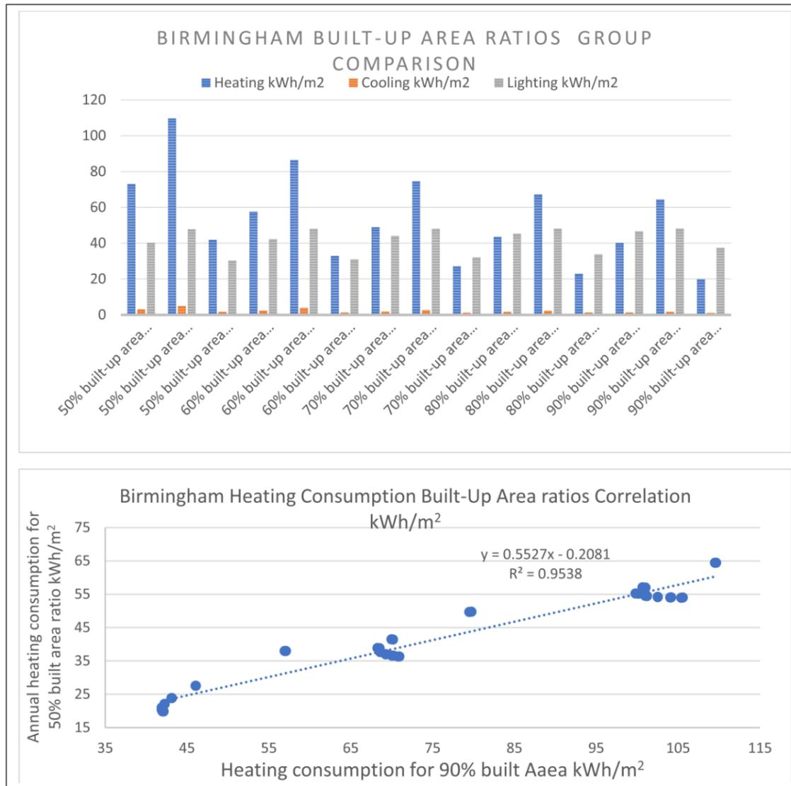
Figure of Built-up area ratio variations' heating consumption average comparison in kWh/m2, built-up area ratio variations' bound correlated in kWh/m2 for Birmingham, UK
