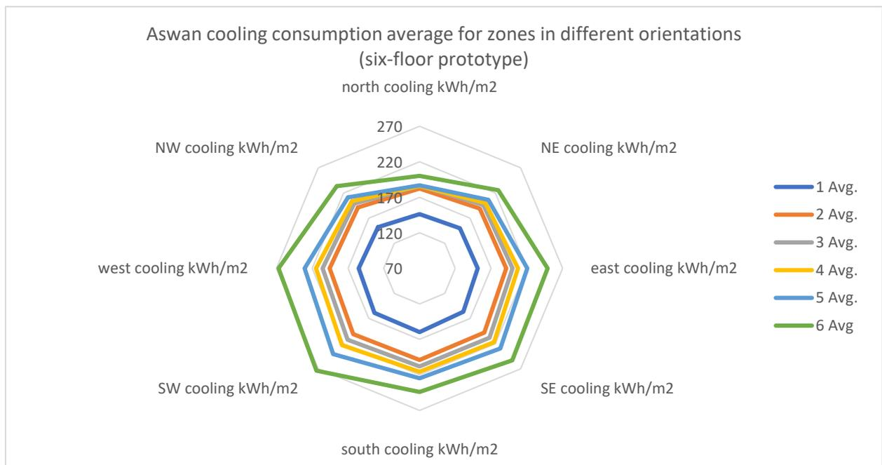
Figure 4-34 Six-floor prototype cooling consumption results average per orientation for Aswan, Egypt
