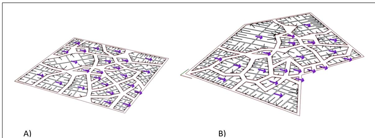
Figure 5-6 Vector X for each urban block and the buildable areas' vectors that help in sorting and tagging each building based on its location in the urban block. A) the first option with typical rectangular boundary and B) a custom-shaped boundary.
