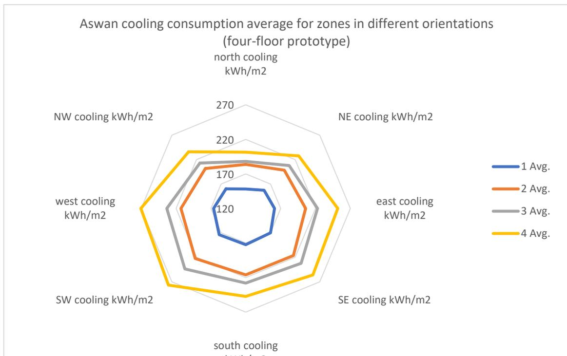
Figure 4-28 Four-floor prototype cooling consumption results average per orientation for Aswan, Egypt
