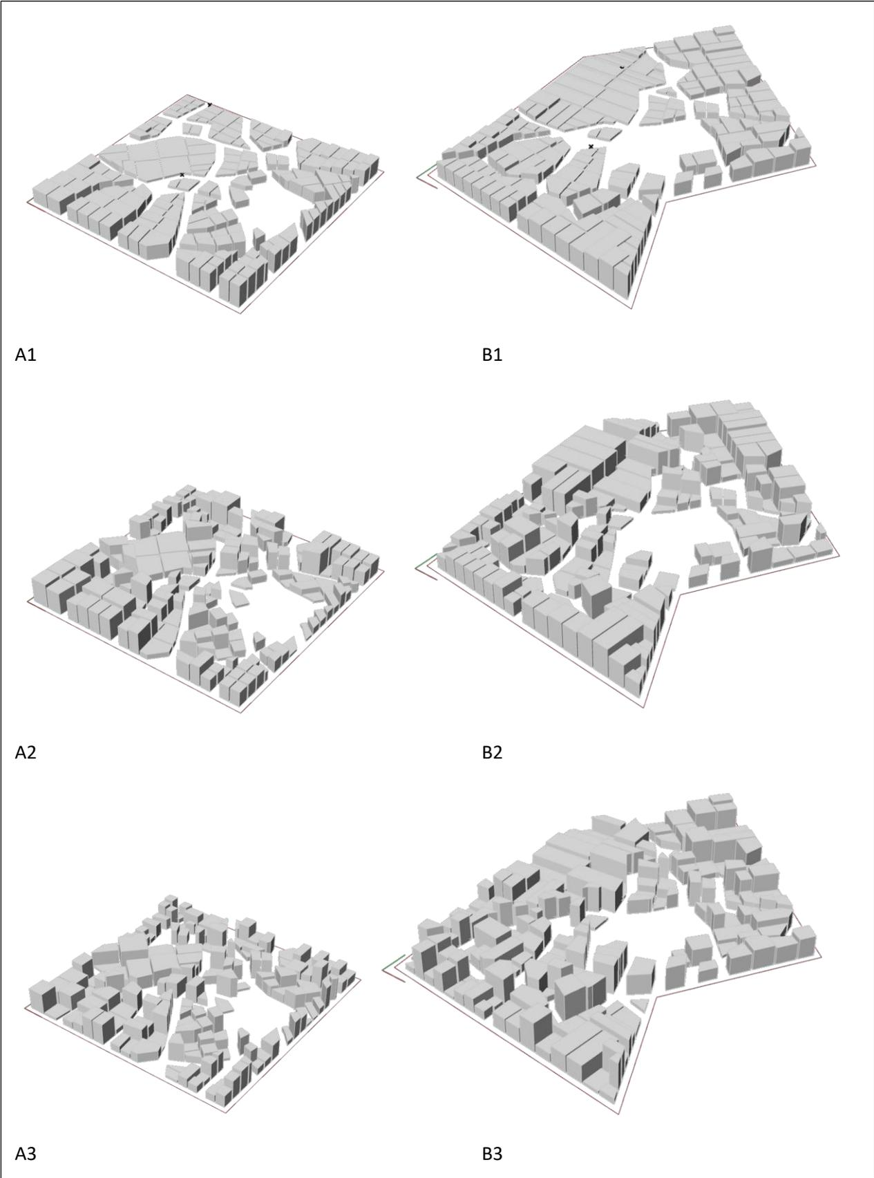
Figure 5-14 Different height option results on the two predefined urban boundaries: A1 and B1 heights by attractor points, A2 and B2 heights by area, A3 and B3 heights by random selection
