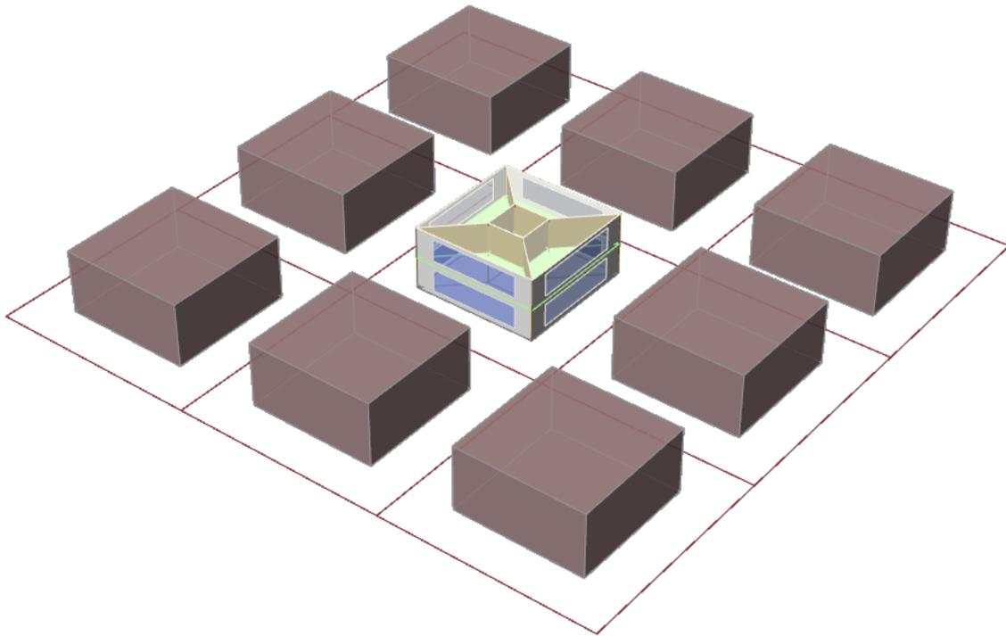
Figure 4-21 Two-floor prototype with 50% WWR and 60% built area ratio and no rotation Iterations with two-floor height had another layer of consumption for the first-floor zones with the eight orientations. For the Aswan cooling demand, the first floor echoes the performance of the ground floor, and both do not show a difference of pattern in consumption from the one-floor prototypes. One important note is that the cooling demand
