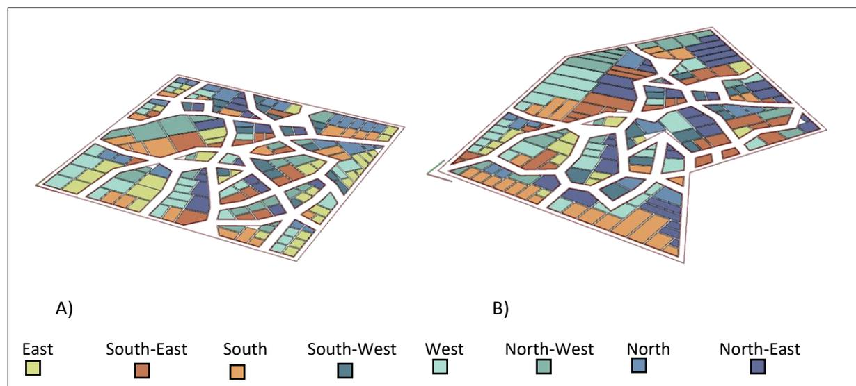
Figure 5-7 Buildable areas colour-coded based on orientation. A) the first option with typical rectangular boundary and B) a custom shape boundary.
