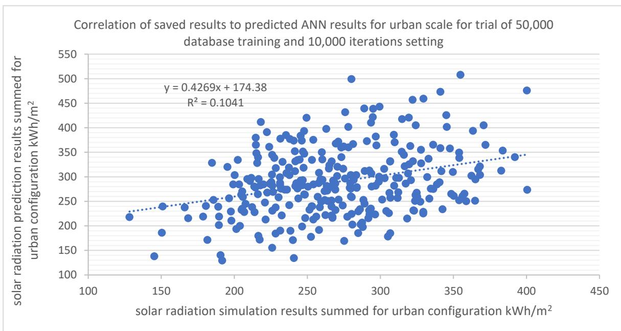
Figure 7-8 Correlation between simulation and prediction results for 300 configurations with ANN trained on 50,000 entries and 10,000 iterations setting
