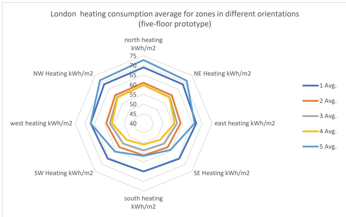
Figure 4-32 Five-floor prototype heating consumption results average per orientation for London, UK
