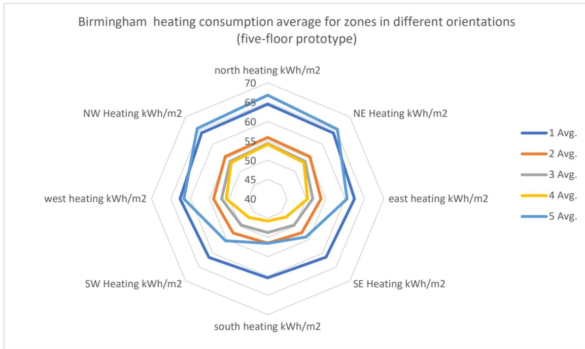
Figure of Five-floor prototype heating consumption results average per orientation for Birmingham, UK
