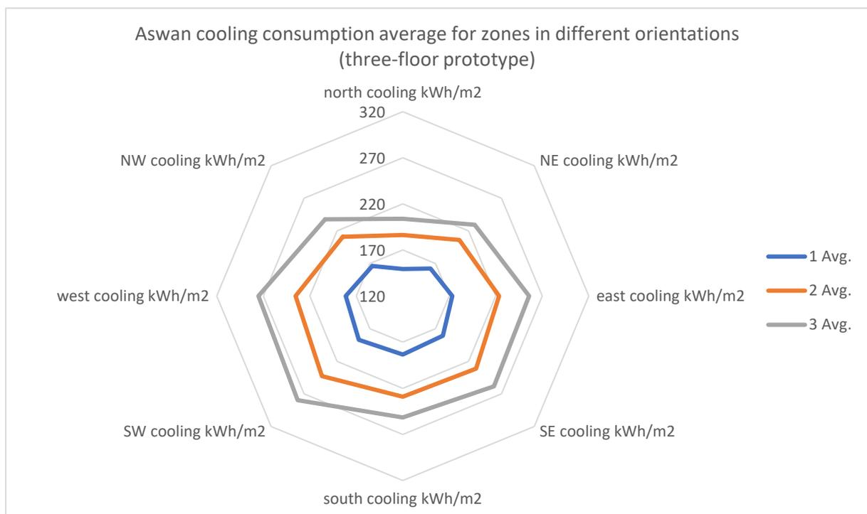
Figure 4-25 Three-floor prototype cooling consumption results average per orientation for Aswan, Egypt
