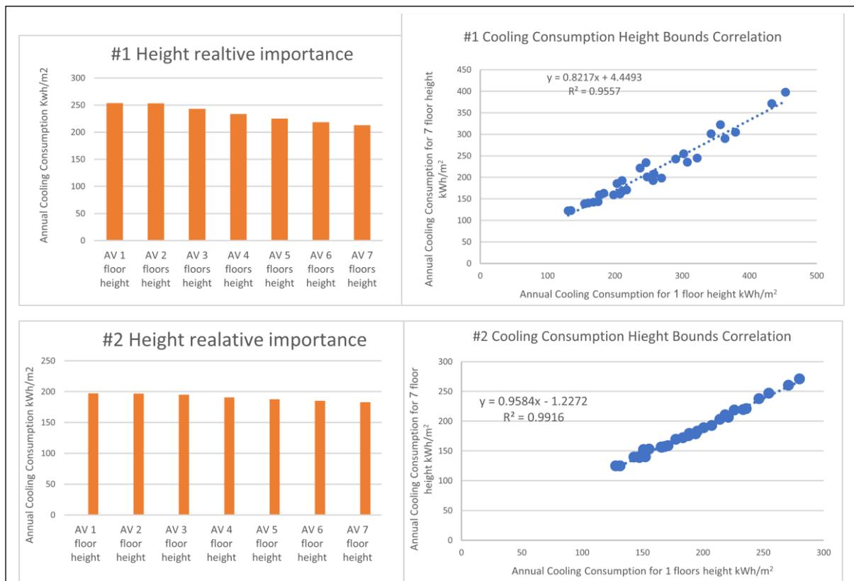
Figure 4-9 (#1) To the left: height variations’ cooling average consumption comparison in kWh/m<sup>2</sup>, to the right: height variations’ bound correlated in kWh/m<sup>2</sup>, (#2) To the left: height variations’ cooling consumption average comparison in kWh/m<sup>2</sup>, to the right: height variations’ bound correlated in kWh/m<sup>2</sup>
