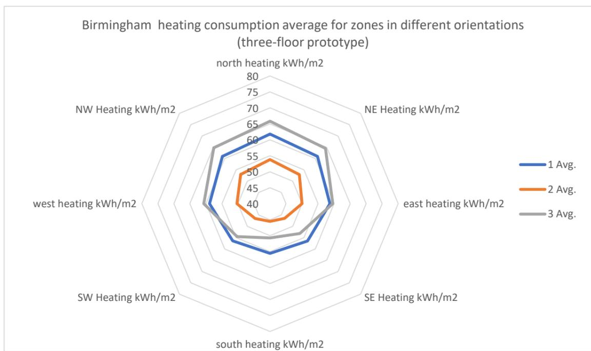
Figure of Three-floor prototype heating consumption results average per orientation for Birmingham, UK
