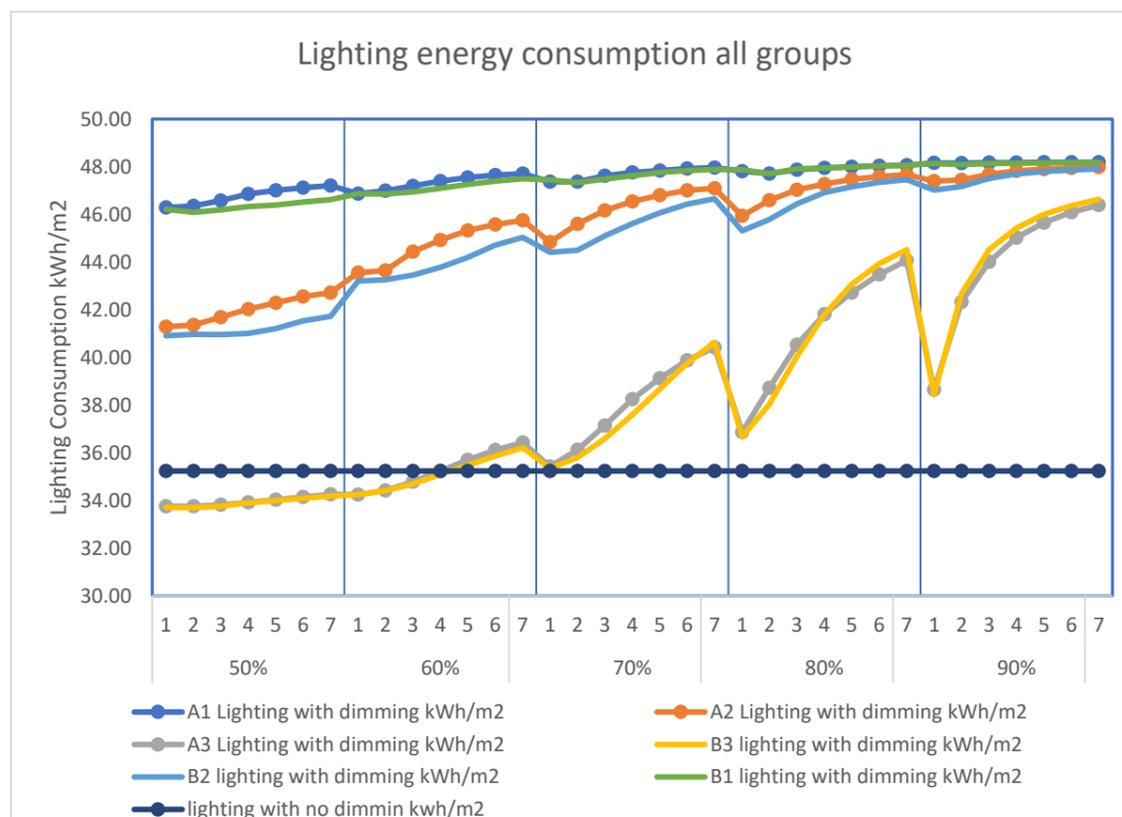
Figure shows the Lighting consumption patterns of the six groups compared with no dimming kWh/m2 results
