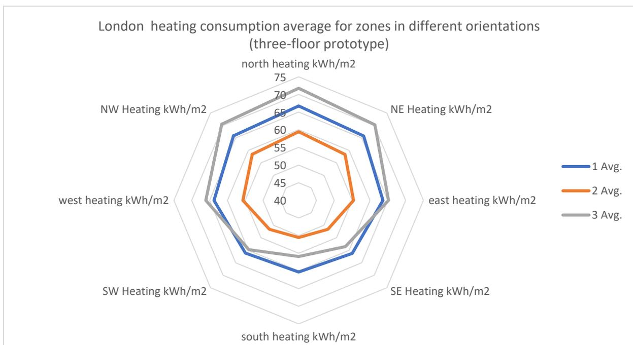
Figure 4-26 Three-floor prototype heating consumption results average per orientation for London, UK
