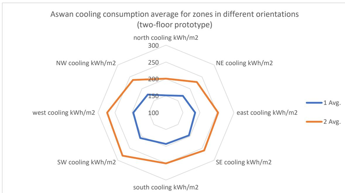
Figure 4-22 Two-floor prototype cooling consumption results average per orientation for Aswan, Egypt
