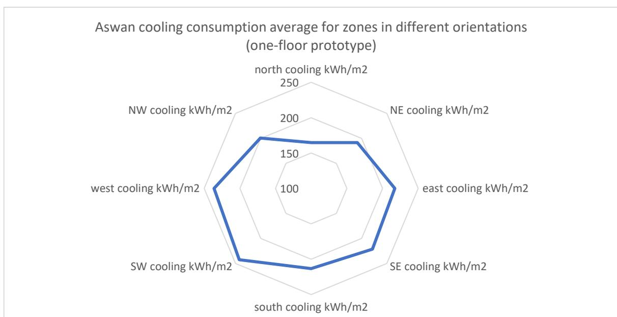
Figure 4-19 One-floor prototype cooling consumption results average per orientation for Aswan, Egypt
