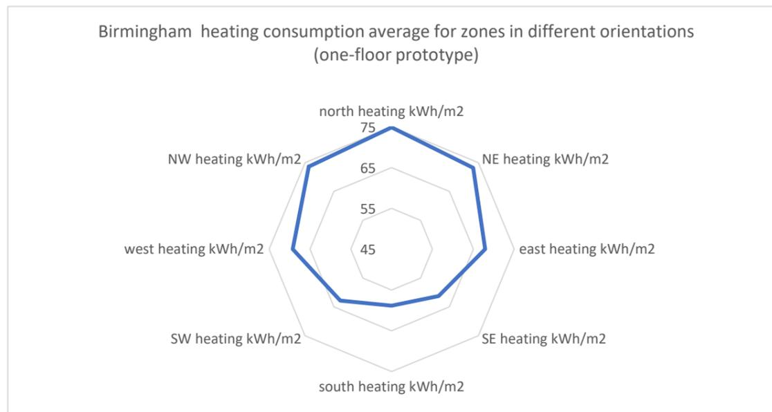
Figure of One-floor prototype heating consumption results average per orientation for Birmingham, UK
