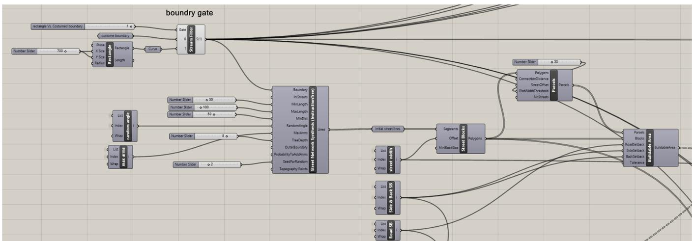
Figure 5-2 The initial input of model's boundary and the gate controlling the two mentioned options. Decoding Spaces used components to generate street networks and buildable areas for the model's initial start
