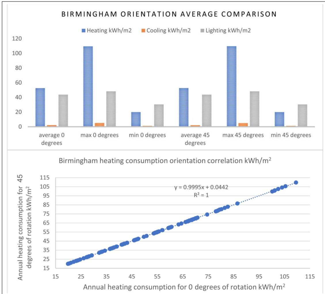
Figure of Orientation variations' heating consumption average comparison in kWh/m<sup>2</sup>, orientation variations' bound correlated in kWh/m<sup>2</sup> for Birmingham, UK
