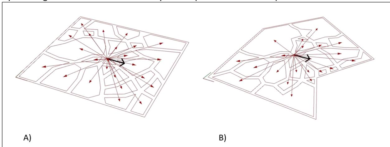
Figure 5-3 The vectors generated by the framework for each block to identify its orientation. A) the first option with typical rectangular boundary and B) a custom-shaped boundary
