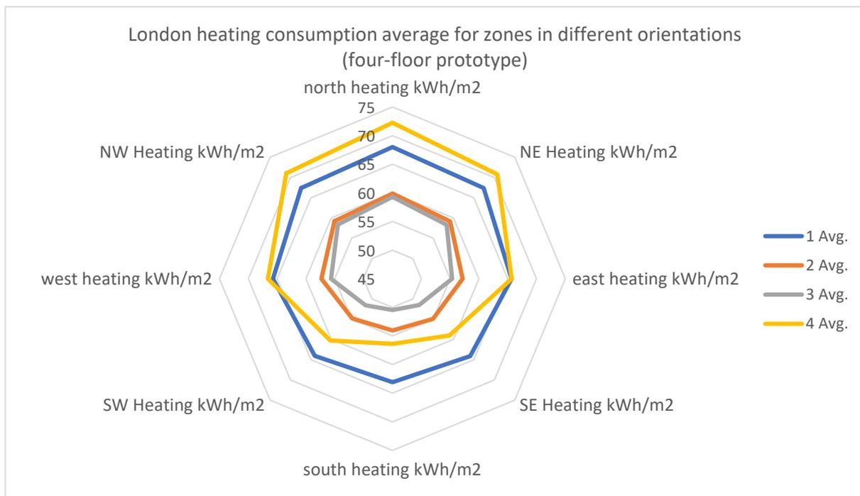
Figure 4-29 Four-floor prototype heating consumption results average per orientation for London, UK
