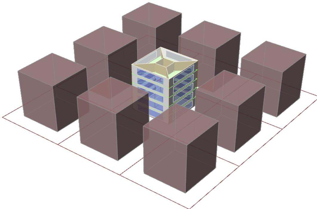
Figure 4-31 Five-floor prototype with 50% WWR and 60% built area ratio and no rotation
