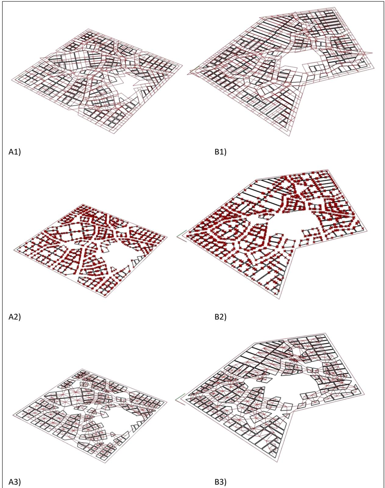
Figure 5-15 Surrounding height comparison different stages. A1 & B1, the buildable areas offsets. A2&B2, shows points of intersections between the offsets and the surrounding buildings. A3&B3,, drawing lines from each buildable area to its surrounding buildings centre points.
