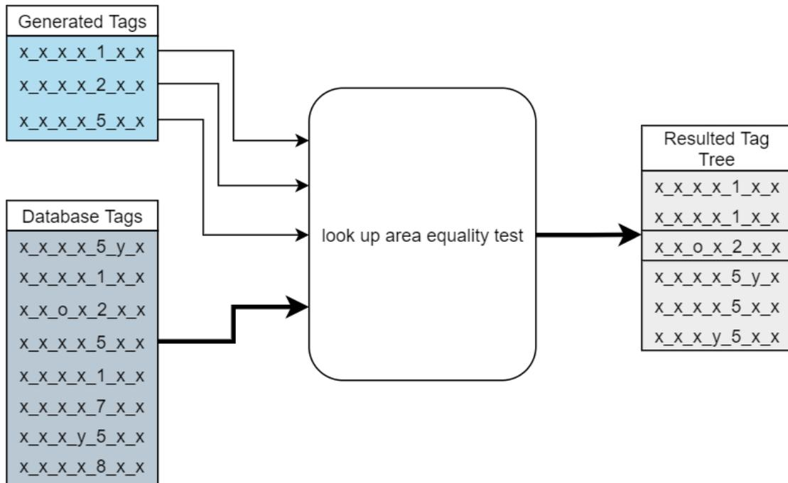
Figure 6-13 Simplified diagram of the tag similarity test
