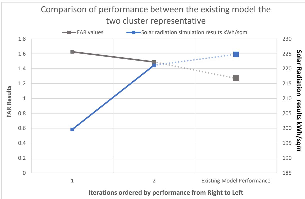
Figure 8-20 Comparison of the fittest 2 representative clusters with the existing model results was conducted for these two cluster representatives to get their actual simulation results. The simulation results are compared with the existing model results in Figure 8-20 and the FAR results. It can be seen that the performance for the two fitnesses are better performing for the two GA selected iterations.
