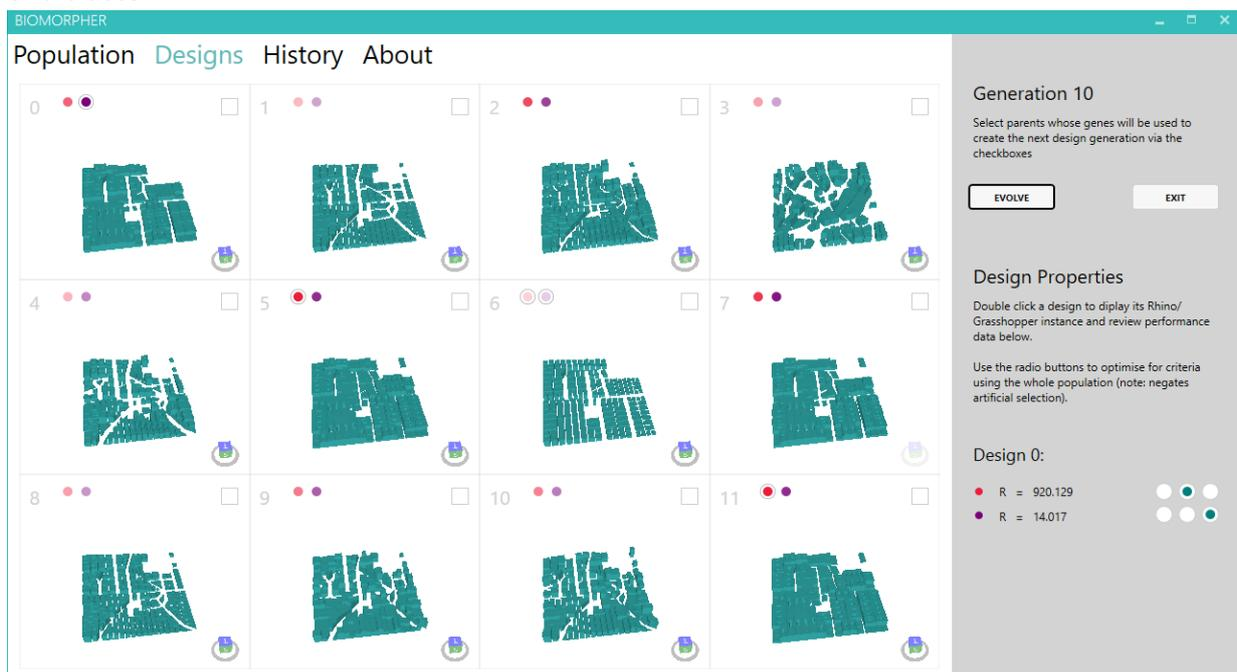
Figure 8-2 The last 12 clusters of the GA 10<sup>th</sup> generation for the 1,000 iteration pool test
