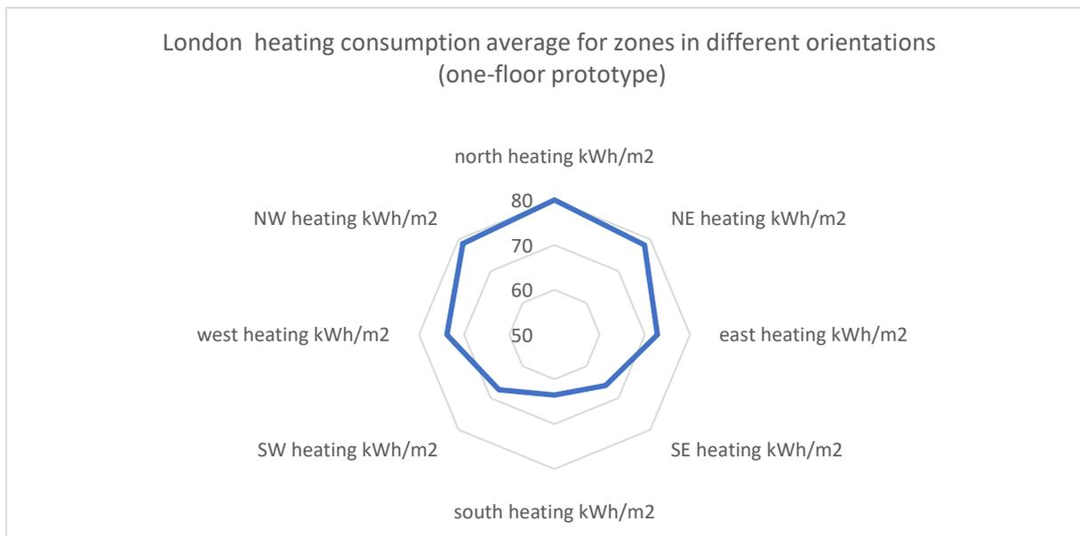
Figure 4-20 One-floor prototype heating consumption results average per orientation for London, UK
