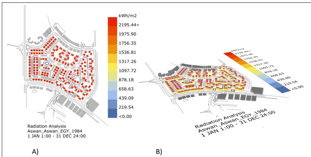
Figure 8-17 Model of simulation results for selected neighbourhood A) the top view of simulation results the existing status of the neighbourhood. B) perspective view for the model results.
