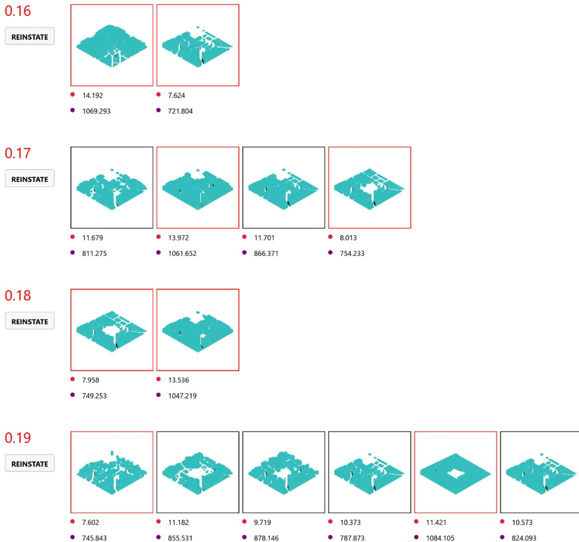
Figure 8-8 The last four generations in the last full database test (red dots for FAR results and blue dots for solar radiation prediction in kWh/sqm)
