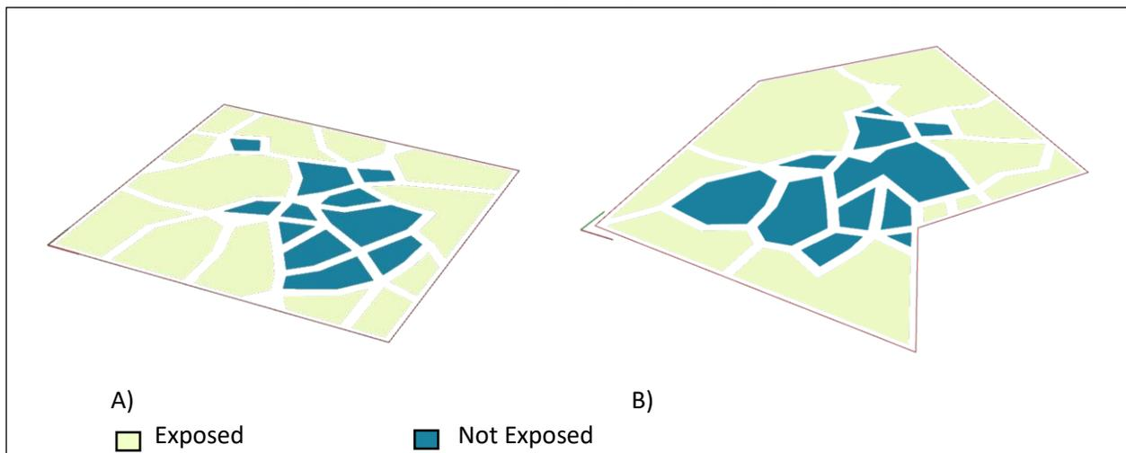
Figure 5-4 Blocks' main street exposure done by the framework sorting. A) the first option with typical rectangular boundary and B) a custom-shaped boundary
