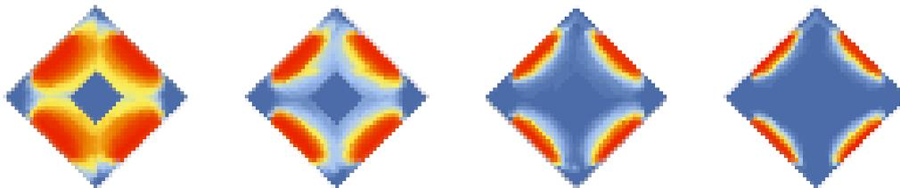
Figure 4-6 Daylight autonomy results illustration for 45 degrees rotation, 20% WWR, 4-floor height and 70% built area ratio showing the results of different zones. The floors order begins with the ground floor to the right up to the 5th floor to the left
