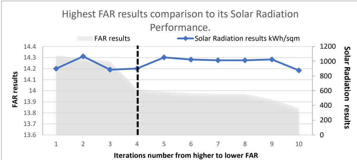
Figure 8-3 Highest 10 FAR values with their solar radiation results and the GA found iteration (in dashed line)
