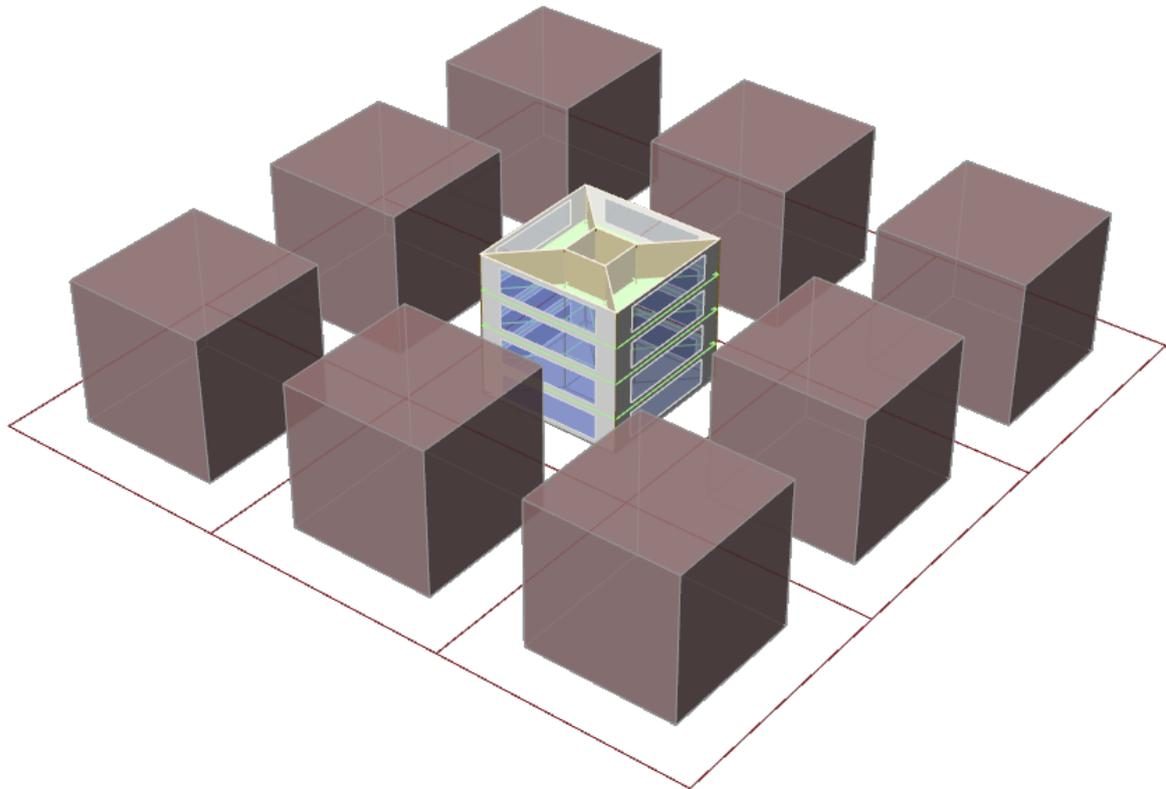
Figure 4-27 Four-floor prototype with 50% WWR and 60% built area ratio and no rotation
