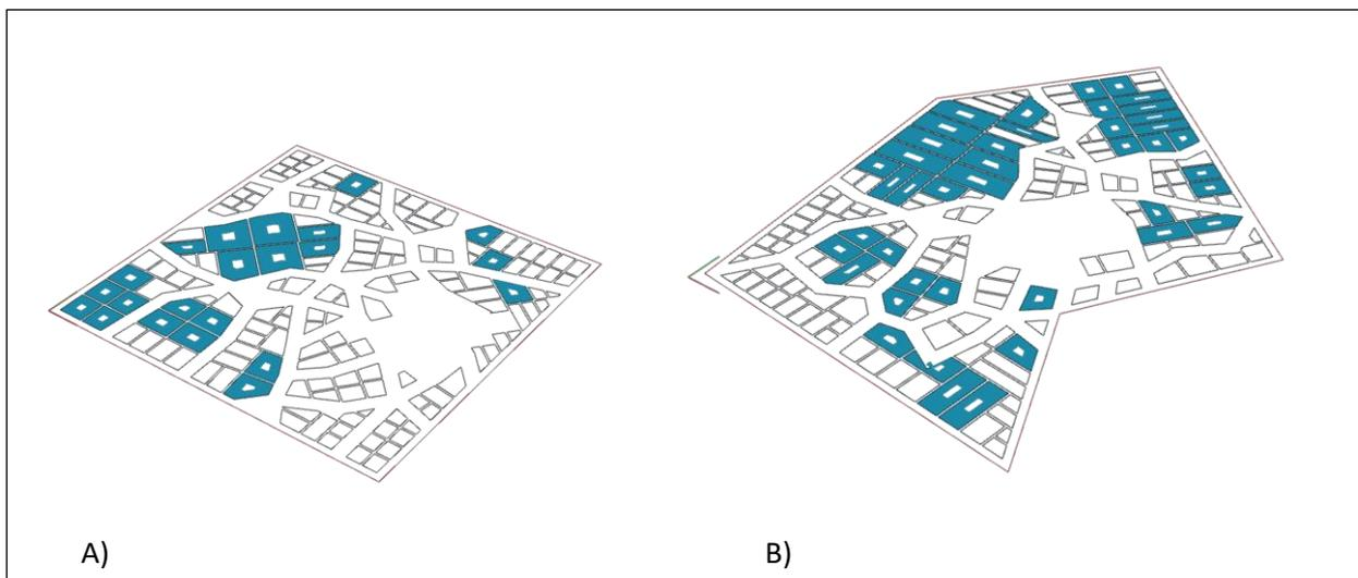
Figure 5-13 Building courts generated for buildable areas that are larger than the preset area threshold the user can control its threshold. For this model, the area threshold is set to 2,500 sq m which means any buildable area larger than this value will have a centric court in it with a scale of 30% of its area, and this ratio is controllable. This allows the user to determine the scale of
