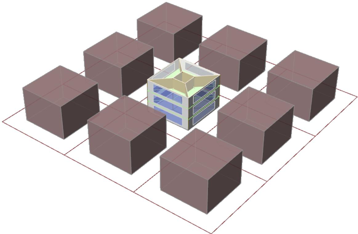
Figure 4-24 Three-floor prototype with 50% WWR and 60% built area ratio and no rotation
