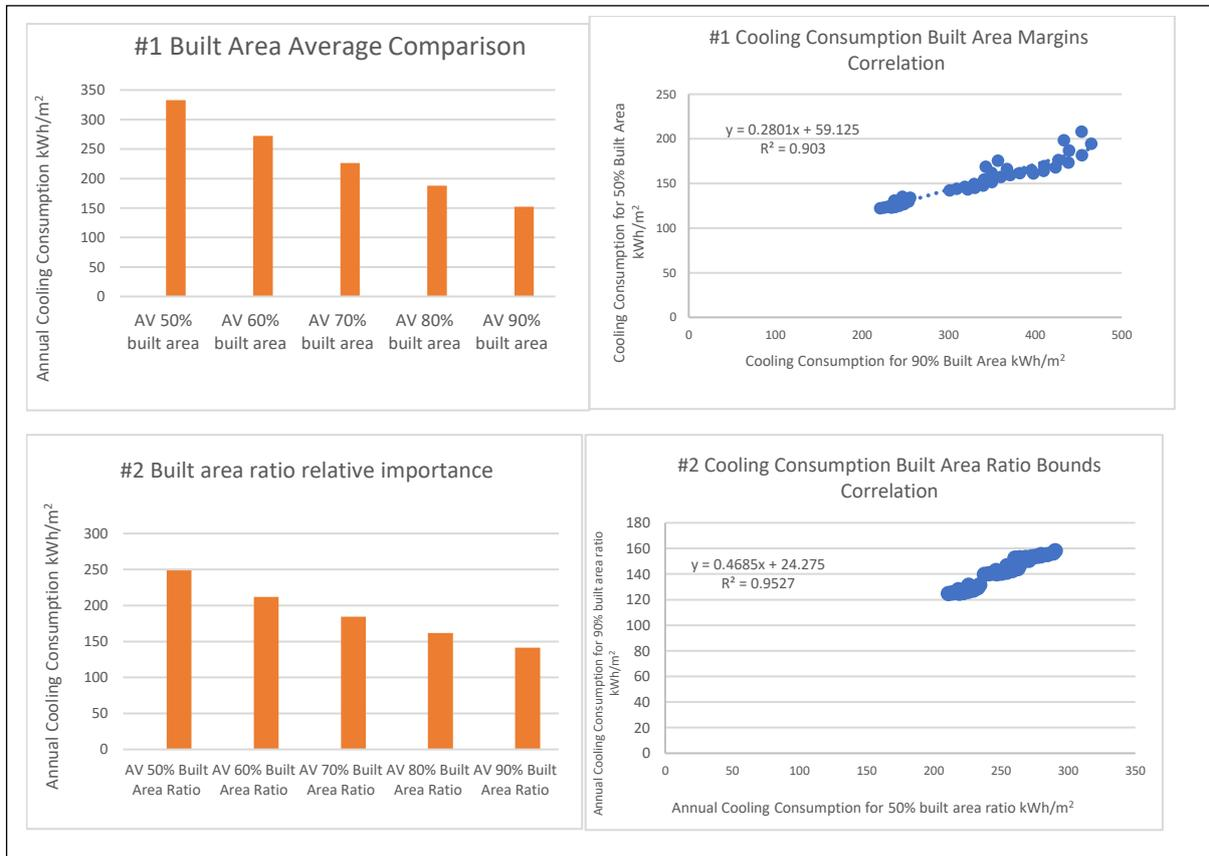
Figure 4-10 (#1) To the left: built area ratio variations' cooling consumption average comparison in kWh/m<sup>2</sup>, to the right: built area ratio variations' bound correlated in kWh/m<sup>2</sup> for the first phase, (#2) To the left: built area ratio variations' cooling consumption average comparison in kWh/m<sup>2</sup>, to the right: built area ratio variations' bound correlated in kWh/m<sup>2</sup> for the second phase
