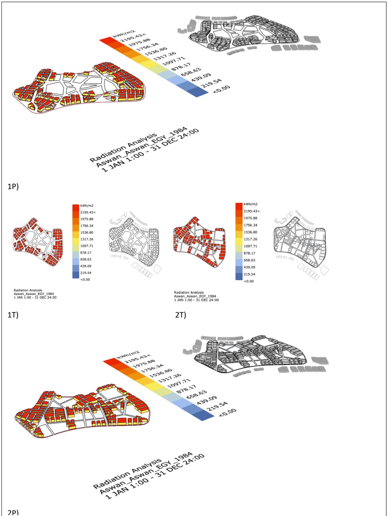
Figure 8-21 Two GA selected models and simulation visualization results shown in perspectives (P) and top views (T) for iterations 1 and 2
