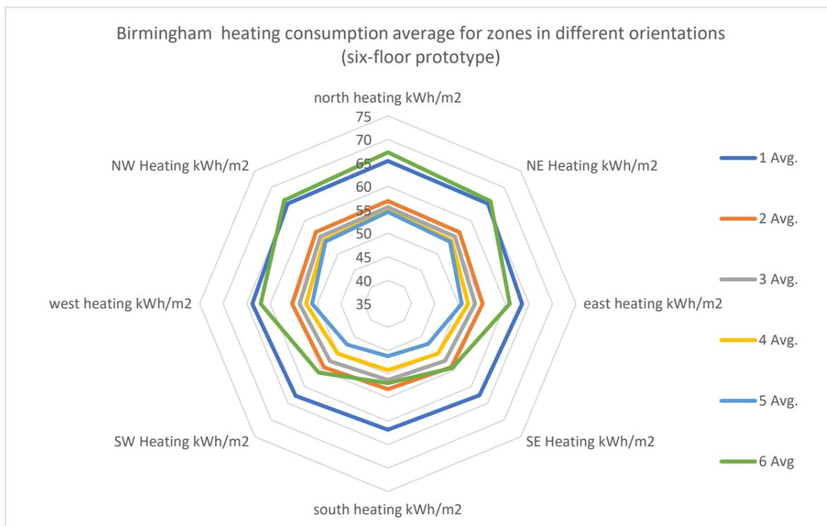
Figure of Six-floor prototype heating consumption results average per orientation for Birmingham, UK
