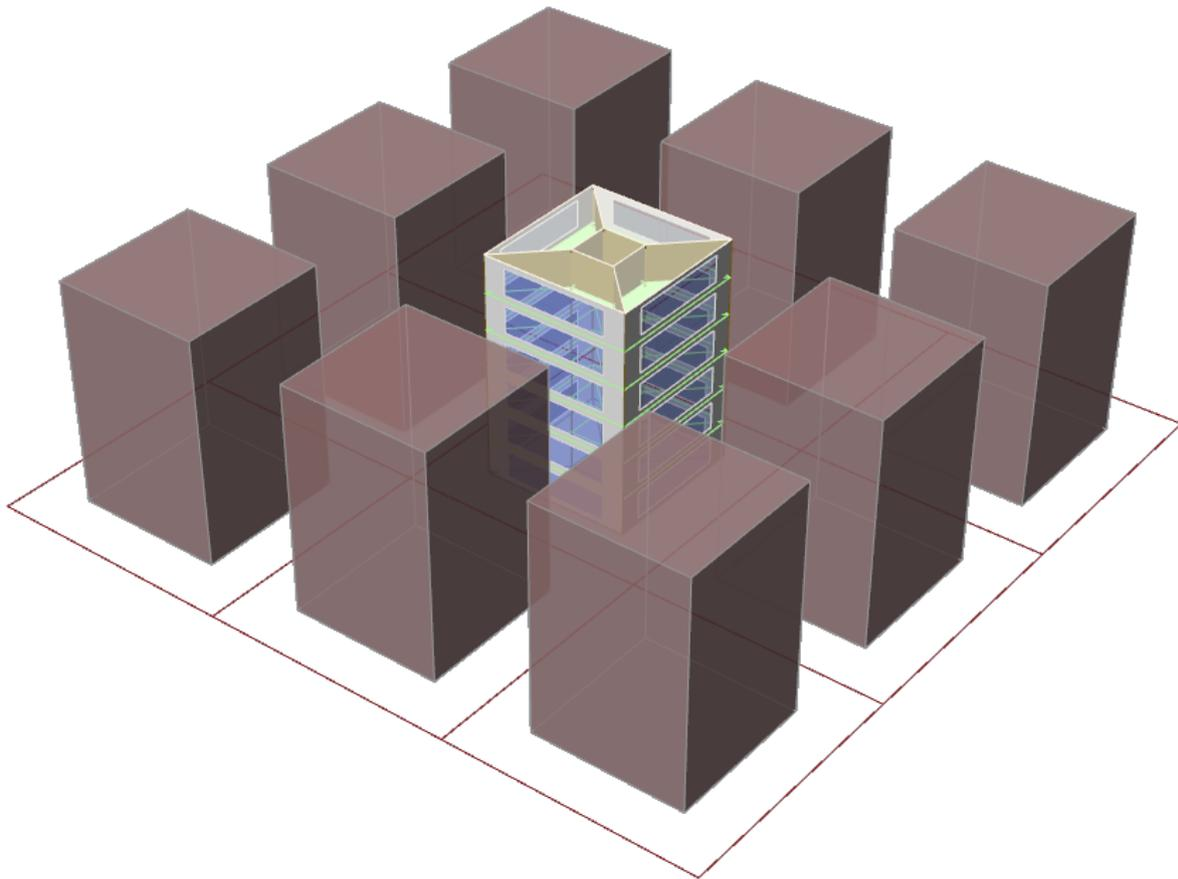
Figure 4-33 Six-floor prototype with 50% WWR and 60% built area ratio and no rotation
