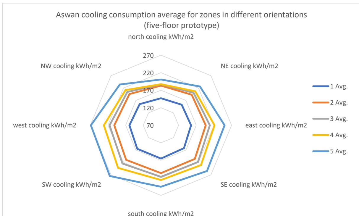
Figure 4-30 Five-floor prototype cooling consumption results average per orientation for Aswan, Egypt
