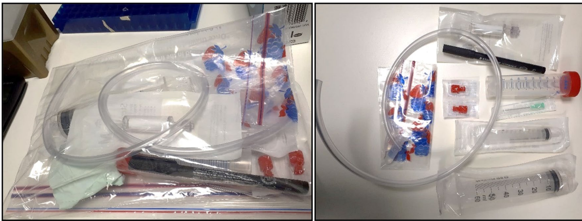
Fig. 1 Images to show the small size of one tree hole eDNA sampling kit. Right, clockwise; Sterivex filter, permanent marker pen, falcon tube, sterile needle, 5 ml syringe, 60 ml syringe, plastic tubing, luer locks and preservation buffer in 5 ml tubes inside a small ziplock bag
