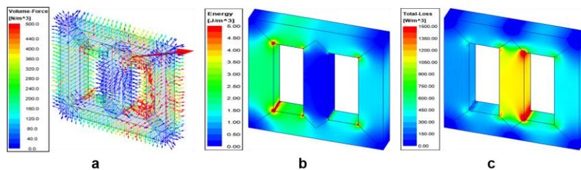
254 **Figure 7. a)** Force distribution **b)** Energy distribution **c)** Total loss distribution for same magnetic flux density
