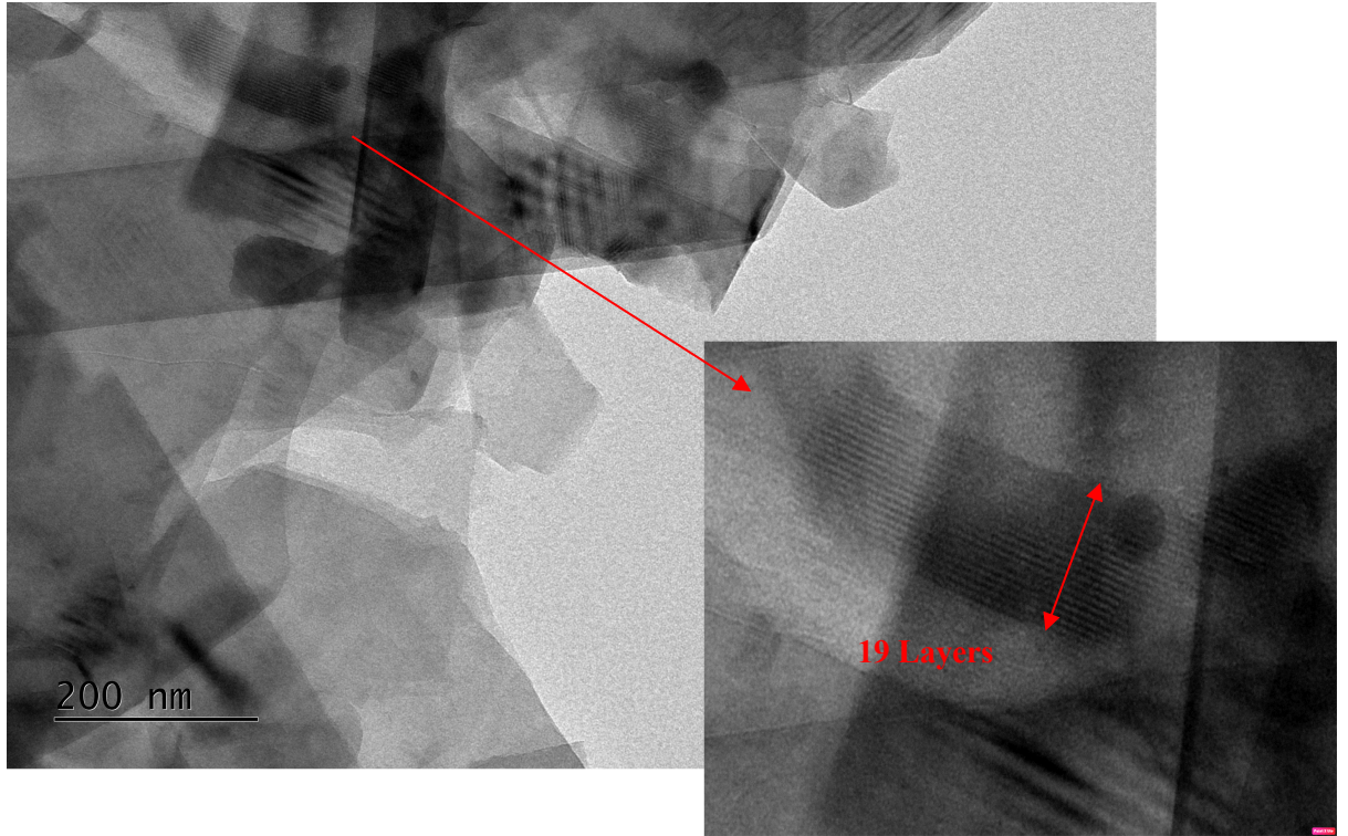
Figure 4.2 : TEM image of GNP-U flake and number of layers in a particulate
