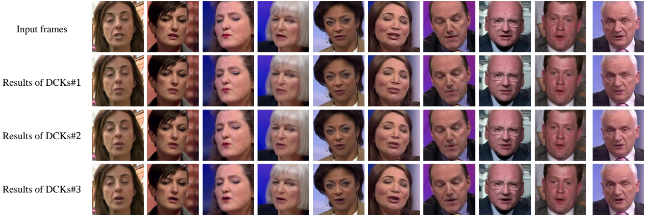
Fig. 6. Given different audio inputs (successive 3 frames of the word ‘for’), our system f' can infer different DCKs (i.e., DCKs#1,#2 and #3), such that f' with DCKs#1,#2 and #3 can transfer a face (with arbitrary expression in any input frame) into expressions with different mouth shapes.
