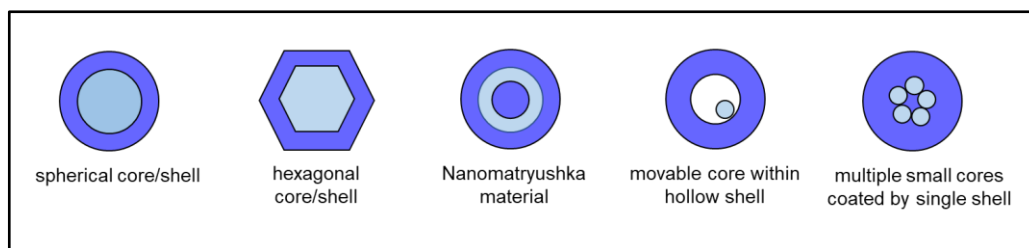
Figure 3.9 Different types of Core-Shell particles. Adapted from R. Chaudhuri et al. 18
