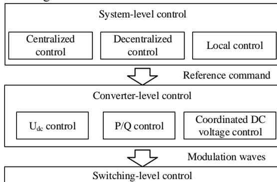
Fig. 3. Control structure of SOPs.
