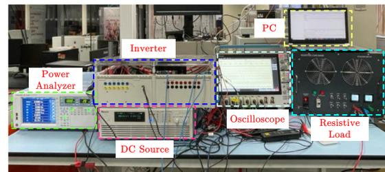
**FIGURE 6.** Experimental setup.
