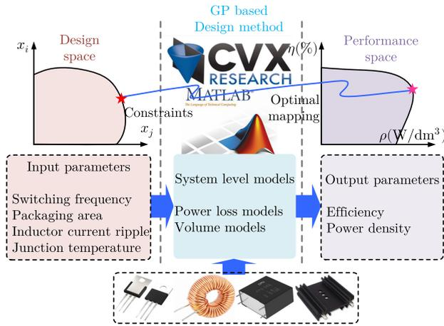
**FIGURE 3.** Overview of multi-objective design using GP.
