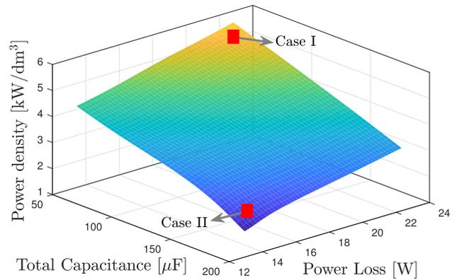
FIGURE 2. Relationship between total capacitance vs. inverter power loss vs. power density.
