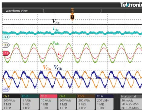
**FIGURE 12.** Steady-state waveforms at 1 kW with second-order ripple controller ( $V_{dc}$ ,  $V_{Ca}$ ,  $V_{Cb}$ : 200 V/div,  $i_{dc}$ : 5 A/div,  $i_a$ : 10 A/div,  $v_{ab}$ :300 V/div).
