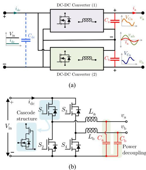
**FIGURE 1.** (a) Single-phase differential inverter with power decoupling function. (b) Buck-type topology under investigation.
