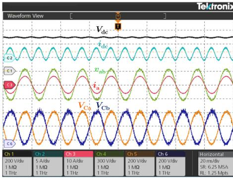
**FIGURE 11.** Steady-state waveforms at 1kW without second-order ripple controller ( $V_{dc}$ ,  $V_{Ca}$ ,  $V_{Cb}$ : 200 V/div,  $i_{dc}$ : 5 A/div,  $i_a$ : 10 A/div,  $v_{ab}$ :300 V/div).
