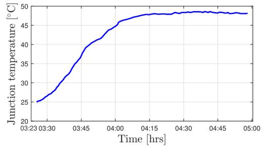
FIGURE 10. Junction temperature of the devices.
