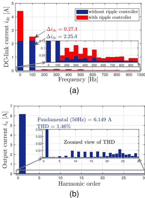
**FIGURE 13.** FFTs of (a) DC-link current with and without second-order ripple controller and (b) output current.
