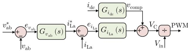
FIGURE 7. Control scheme of the inverter.
