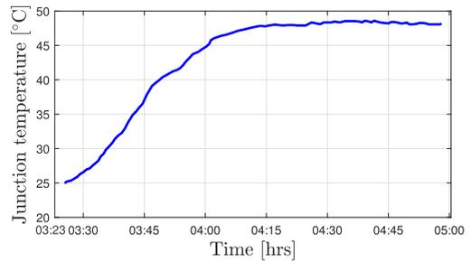
FIGURE 10. Junction temperature of the devices.
