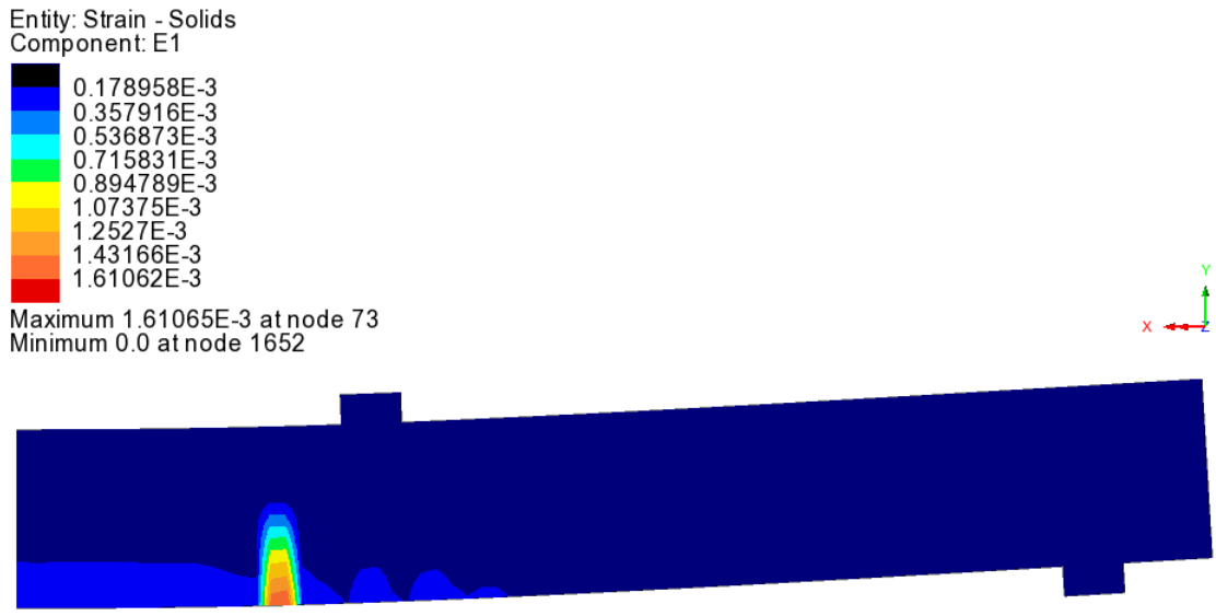
Figure 7.19: Major principal strain profile at stage b in Figure 7.15.
