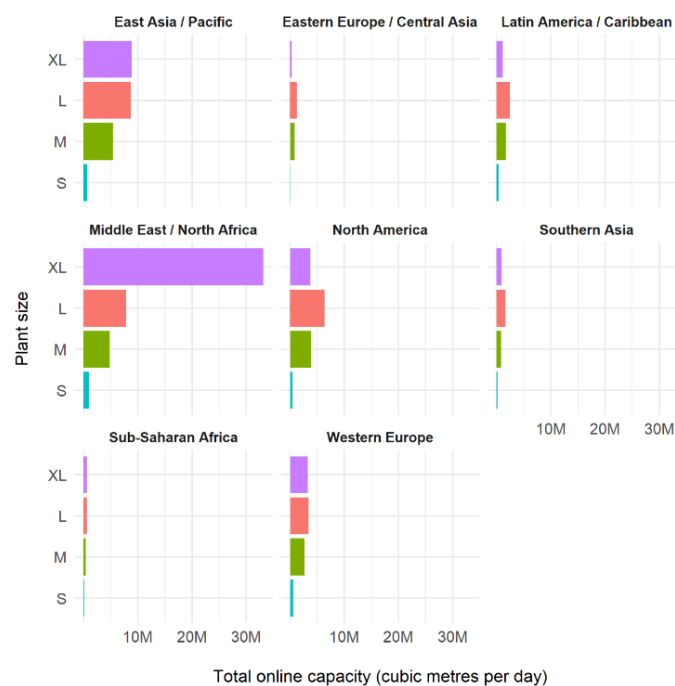
Figure 5. Online and presumed-online desalting capacity in each macro-region, categorised by plant size.
