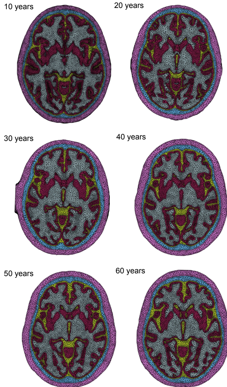
Figure 4.3: Axial views of the generated finite element head meshes for each head atlas, 10-60 years, respectively, visualised using Matlab (Natick, USA). The five head tissues are represented for the scalp (purple), skull (blue), CSF (yellow), GM (pink) and WM (grey). The 10-year-old model consisted of 3.8M tetrahedra of size 1\text{mm}^3 and 6.81 \times 10^5 nodes. The 20-year-old model had 3.33M tetrahedra and 6 \times 10^5 nodes. For the 30-year-old mesh, there were 3.35M tetrahedra and 6.14 \times 10^5 nodes. The 40-year-old model contained 3.41M tetrahedra and 6.25 \times 10^5 nodes. For the 50-year-old mesh, there were 3.42M tetrahedra and 6.25 \times 10^5 nodes. Lastly, the 60-year-old model consisted of 3.38M tetrahedra and 6.21 \times 10^5 nodes.
