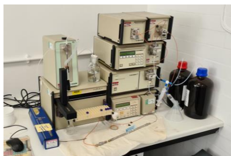
Figure 20: HPLC apparatus used to measure enantiomeric excess of products
