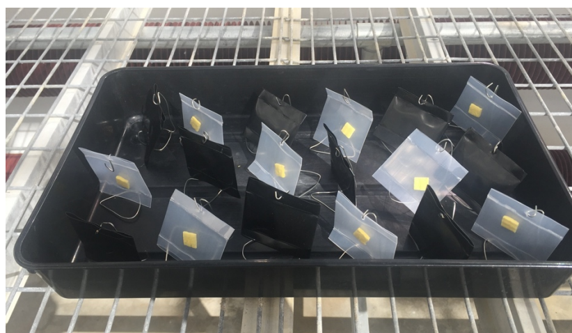
Figure 6.6: Experimental set-up for stability study where black and clear PVC sachets containing yellow sponges dosed with germacrene D are suspended from wire frames and exposed to air and light in a greenhouse environment.
