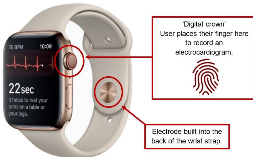
Figure 1.10: Apple Watch Series 4. To record cardiac activity user, place their finger on the digital crown as highlighted in the Figure. Image adapted from Sampson (2019).
