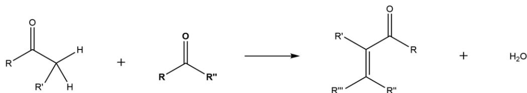
**Figure 5. Simple aldol condensation scheme**
