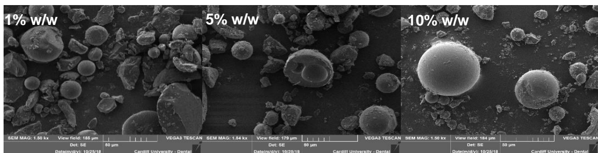
Figure 88: SEM images of gentamicin sulfate and magnesium stearate powder blends of concentration 1% w/w, 5% w/w and 10% w/w with respect to gentamicin sulfate, prepared by manually grinding with a mortar and pestle. Sample magnifications are 1.5k.
