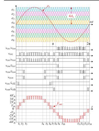
Fig. 3 PD-PWM method schematic
