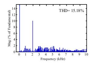
Fig. 7 THD of the output voltage
