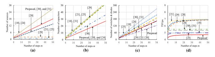
Fig. 5 Comparison of different SCMLIs. a number of sources; b number of capacitors; c number of switches and diodes; d TSV<sub>pu</sub>
