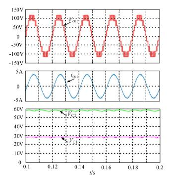
Fig. 6 Simulation results of output voltage, load current, and capacitor voltage
