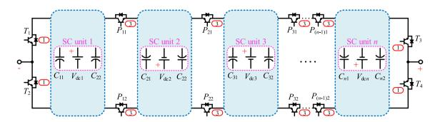
Fig. 4 Extended structure of the proposed 9LSUI
