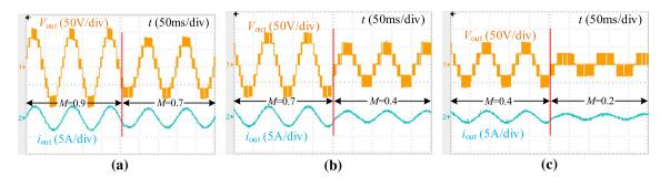
Fig. 11 Dynamic experimental results with change of a M from 0.9 to 0.7, b M from 0.7 to 0.4 and c M from 0.4 to 0.2
