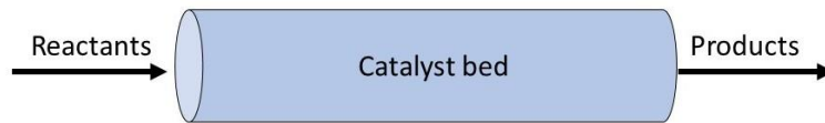
Figure 19 Schematic representation of a lab scale packed bed tubular reactor. The reactants are continuously fed through a tubular reactor packed with a fixed mass of catalyst. Passing through the catalyst bed the reactants are continuously converted in the reaction products, that in turn leave the reactor as effluents.
