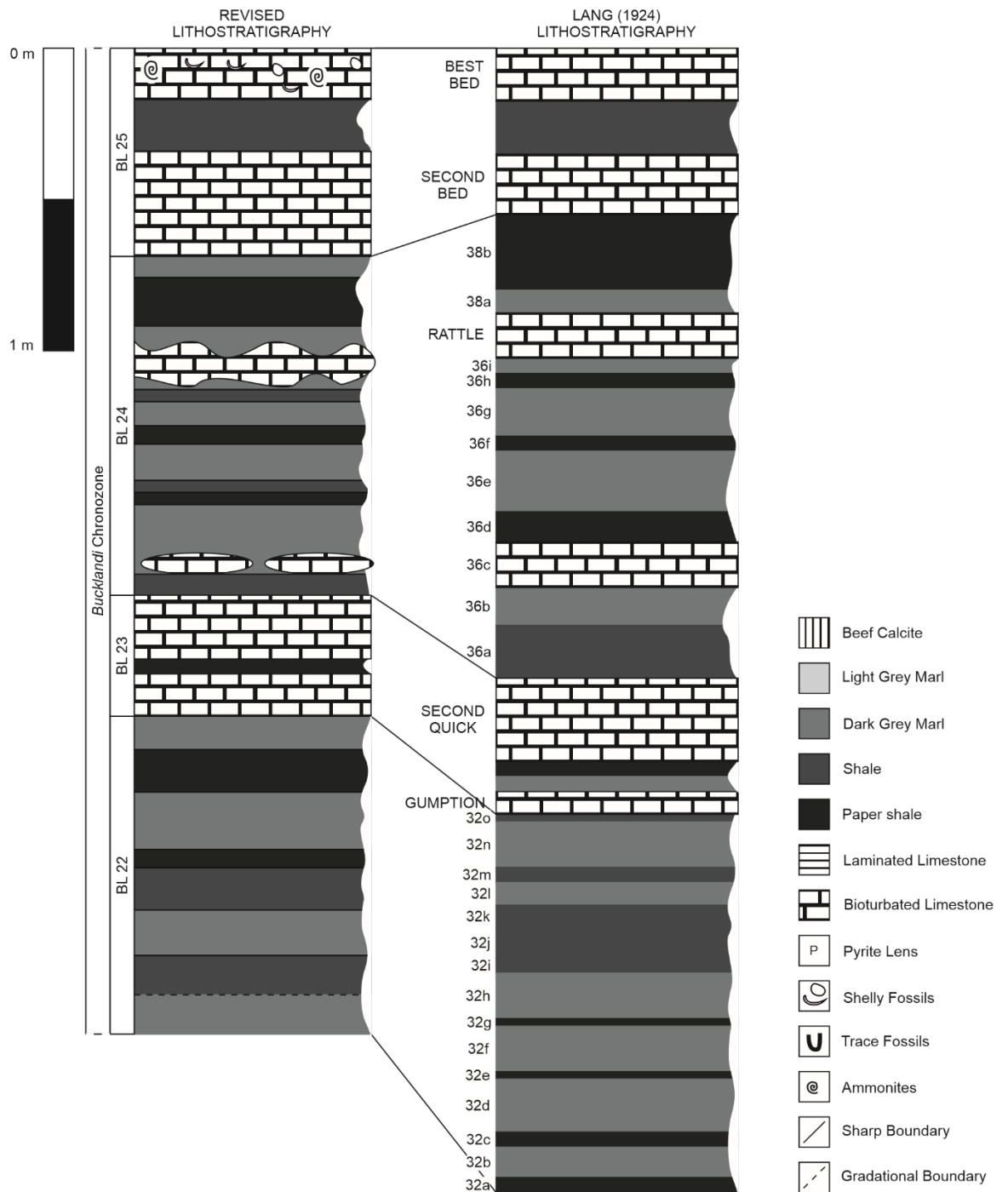
Figure 2.21 – Revised lithostratigraphy of BL 22 – BL 25. Comparison is offered to the lithostratigraphic log of Lang (1924). Key in figure. Scale = 1 m.
