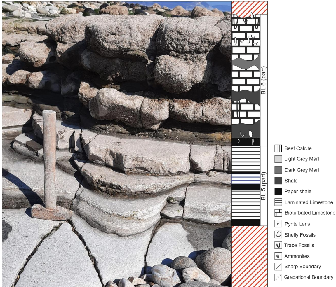
Figure 2.12 – A photograph of BL 5 (part) and BL 6 (part) in Pinhay Bay, Devon (fig. 2.3) to illustrate the contrast between planar laminated limestones and irregular bioturbated limestones. Note the various argillaceous interbeds which include paper shales, shales, and dark marls. There is an additional lenticular laminated limestone highlighted in blue that was laterally limited and therefore not included within the revised lithostratigraphic log (fig. 2.11). Moderate lateral variability in the thicknesses of different beds and the perspective of the image mean that the section shown here may vary from the revised lithostratigraphic log (fig. 2.11). Size of hammer = 350 mm.
