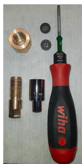
Fig. 2. Setup for making equal volumes of filter media.
