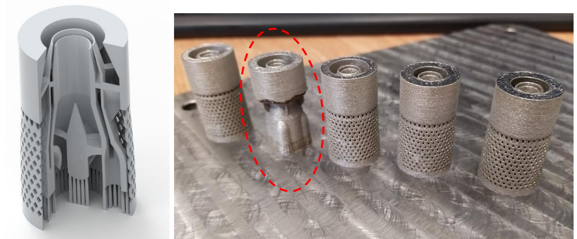
Figure 4-16 - Phase II atomiser manufacturing technique (failed atomiser highlighted)
