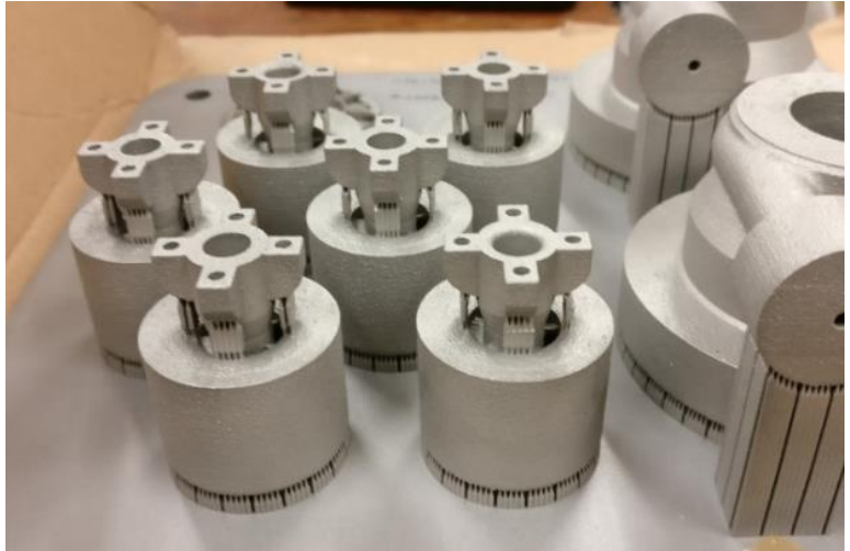
Figure 4-12 - Phase I atomiser manufacturing CAD file with supports (left) and printed atomisers (right)
