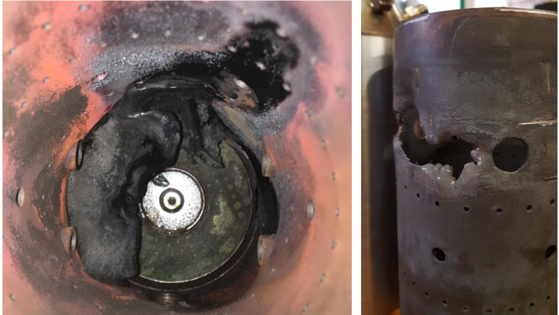
Figure 6-22 - Primary zone nvPM buildup (left) and thermal damage to the liner (right)
