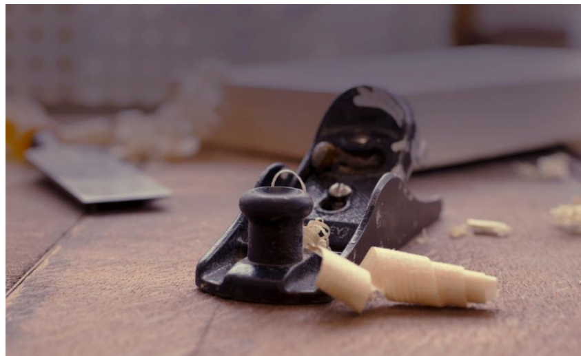
Figure 2.6 Continuous chip formation of wood (Stock Image)
