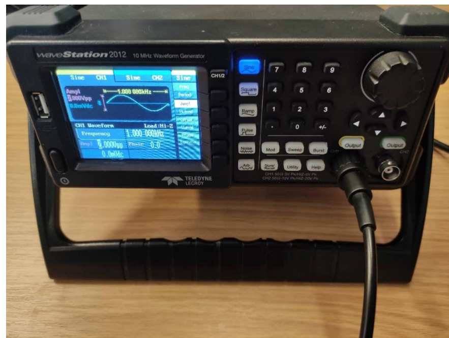
Figure 5.10 Signal Generator producing 1 KHz frequency and 2 V amplitude
