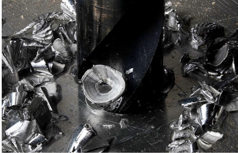
Figure 2.7 Chip formation in steel (JJ Harrison 2008)
