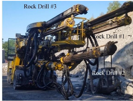
Fig.7 Jumbo at a construction site [47]
