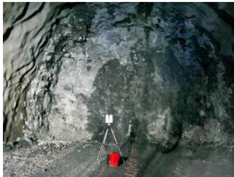
273 Fig.6 LiDAR scanning of a tunnel face with a diameter of 10m in Oslo, Norway [41].
