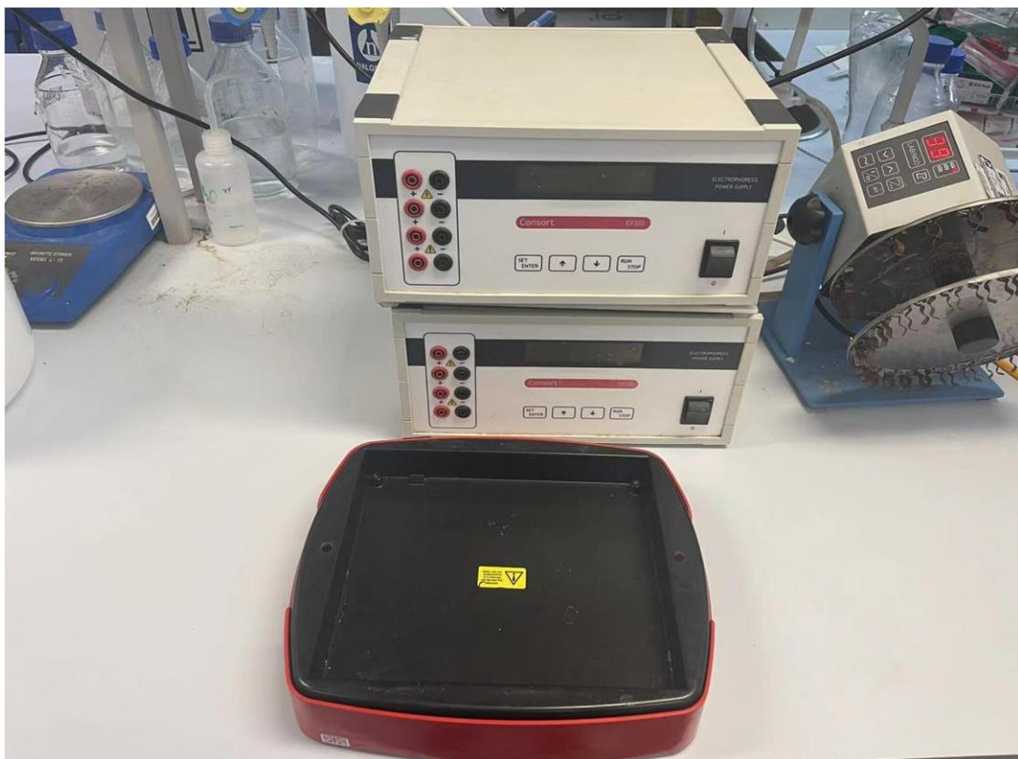
Figure 2.10 SD10 SemiDry Maxi System blotting unit (Wolf Laboratories, York, UK)
