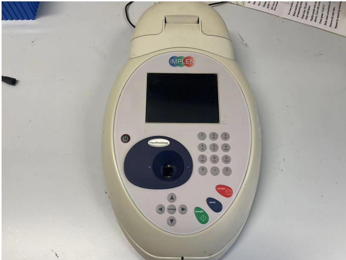
Figure 2.5 IMPLen NanoPhotometer (Geneflow Ltd., Litchfield, UK)
