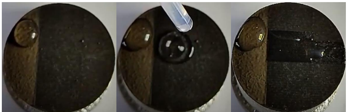
Figure 5.17. Top view of the wettability test.
