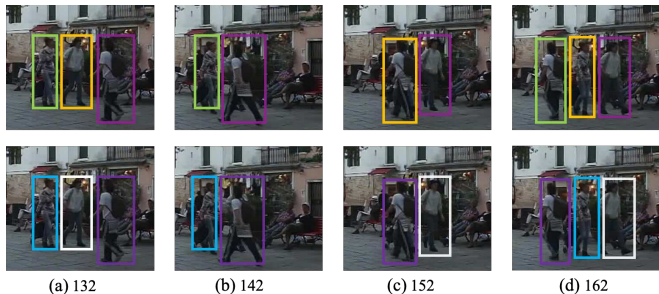
Fig. 5. Visualization of the qualitative results with tube re-assignment. The results are from frames 132, 142, 152, and 162 of sequence MOT17-01. Top row: The results without tube re-assignment make identity association with regression, resulting in ID switches when severe occlusions exist. Bottom row: With tube re-assignment, the motion cues are considered. Thus the identities are assigned correctly.
