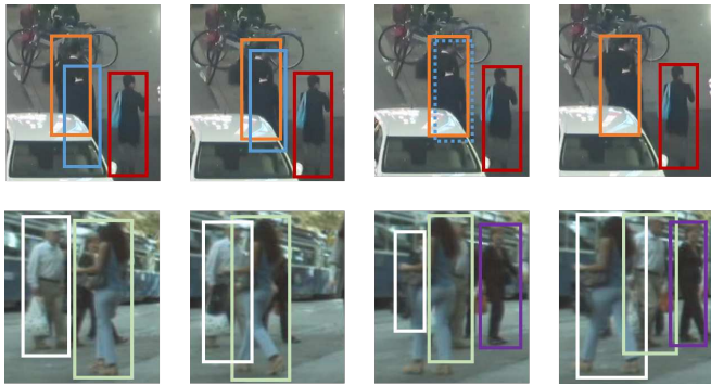
Fig. 1. Noisy features from nearby cause typical false negatives and ID switches in the tracking-by-regression paradigm. The dashed box represents the raw regressed result, which becomes invalid in the post-process. Top row: The nearby targets with similar appearances introduce noisy features. Therefore the dashed blue box drifts to a nearby target and is eventually eliminated. Bottom row: The two boxes in white and green contain mixed features of two targets, and representative features are contaminated as the two targets get closer, resulting in an ID switch. Different box colors indicate different identities. Best viewed in color.
