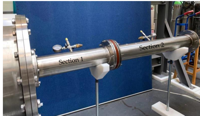
Figure 4. Two installed sections of the constructed GIL prototype separated by the spacer.
