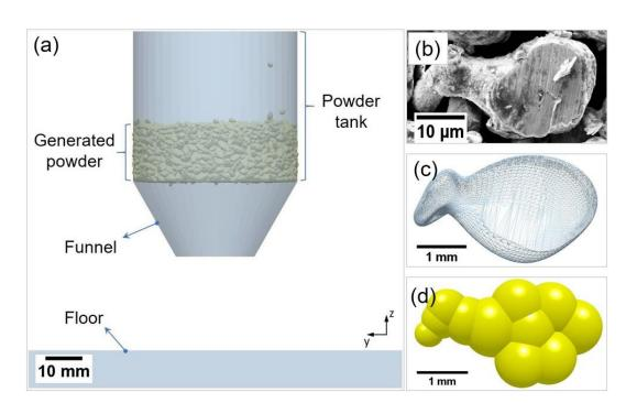
**Figure 2.** Projection of (**a**) simulation model with an example of (**b**) SEM image of the 0.5 h milled powder, (**c**) created a 3D template based on the SEM images of the real powder and (**d**) created DEM particle with 11 spherical cells from the template.
