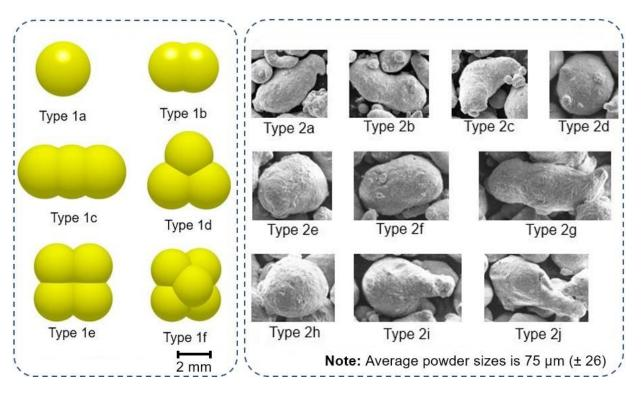
**Figure 3.** Commonly used particle morphologies in literature (Type 1 series) and the most representative particles for SEM photos of the real powders (Type 2 series).
