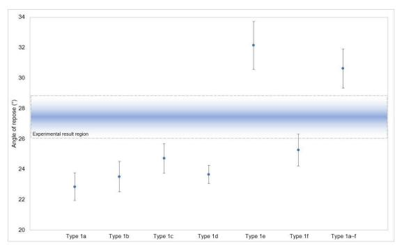
Figure 13. Angle of repose of commonly used particles (Type 1) in the literature.
