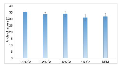
**Figure 19.** The hillside angles of 4 h milled powders with different percentages of Gr (0.1, 0.2, 0.5, and 1 wt.%) and DEM.
