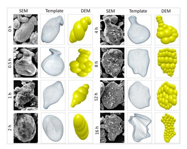
**Figure 4.** Examples of created 3D particles showing the morphological evolution of particle shape from spherical to flat with increasing milling time.
