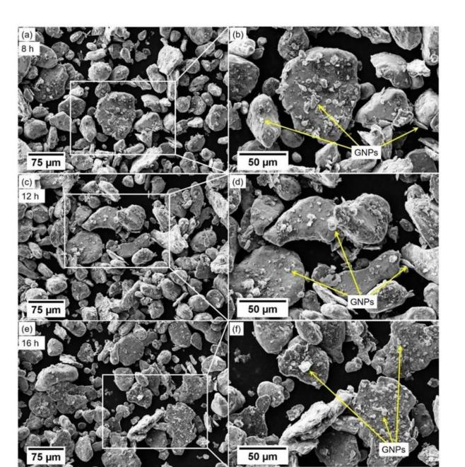
**Figure 8.** SEM images showing the morphological alteration of powders and the dispersion of agglomerated GNPs in the milled alloys for (**a**,**b**) 8 h, (**c**,**d**) 12 h and (**e**,**f**) 16 h with magnified images.
