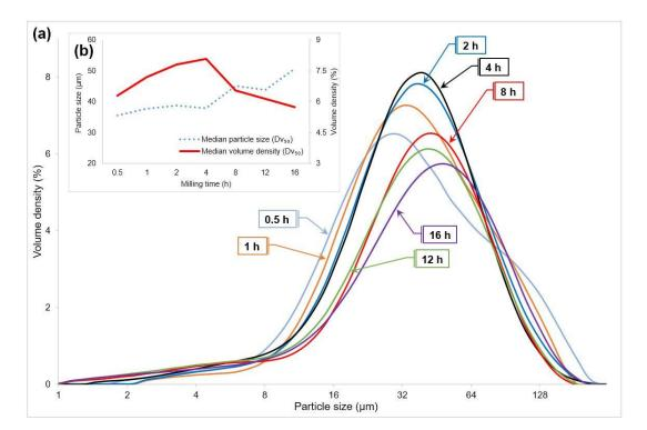
Figure 5. The plot of (a) PSD and (b) median values of milled composites from 0.5 to 16 h.
