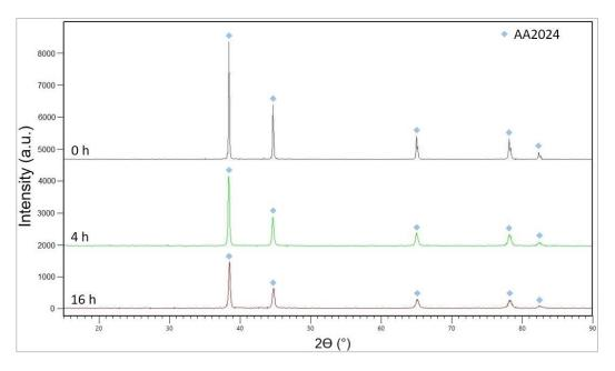
Figure 6. XRD patterns of 0, 4 and 16 h milled composites.
