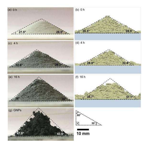
**Figure 17.** Reposed powder, showing GNPs, 0, 4 and 16 h milled alloy from (**a**,**c**,**e**,**g**) experimental work and (**b**,**d**,**f**) DEM simulation.
