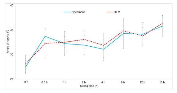
**Figure 16.** Angle of repose of the as-received powder and milled Gr/AA2024 obtained from experimental work and DEM simulation.
