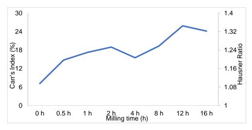
Figure 18. Carr's index and the HR of the composites at different milling times.
