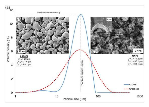
**Figure 1.** (a) The PSD of the alloy and Gr, (b) SEM images of the as-received (0 h) powder and (c) GNPs.
