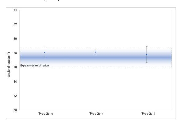
**Figure 15.** Angle of repose of three (Type 2a–c), six (Type 2a–f), and ten (Type 2a–j) powder morphology obtained from SEM images of real particles.
