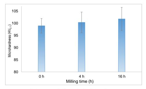
Figure 11. Microhardness test results of 0, 4 and 16 h milled powders.
