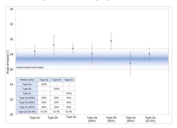
ered, three-particle morphology was representative enough and gives adequate results in comparison to the six and ten morphologies.
