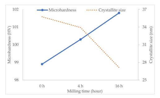
Figure 20. Inverse correlation of microhardness and crystallite size via increasing milling time.
