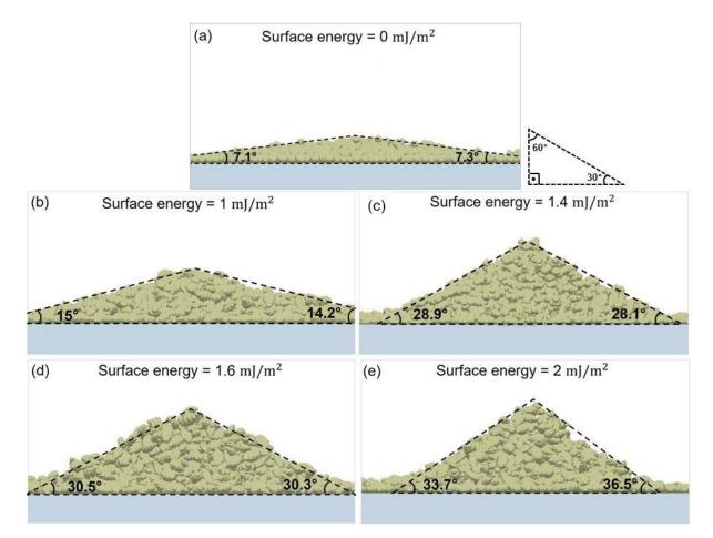
**Figure 12.** The hillside angle of the as-received powder under surface energy values of (**a**) 0, (**b**) 1, (**c**) 1.4, (**d**) 1.6 and (**e**)  $2 \text{ mJ/m}^2$ .
