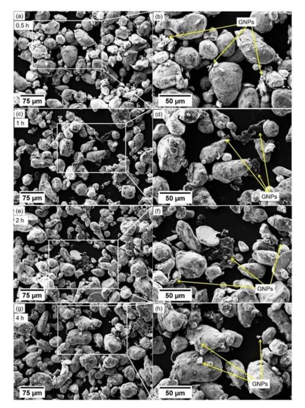
$\pi$ - $\pi$  interaction of Gr [15]. Short milling times promote the formation of agglomerations to begin with, resulting in the impact energy being used to dissolve the Gr particles first. Because of this, shorter milling times tend to result in fewer morphological changes.
