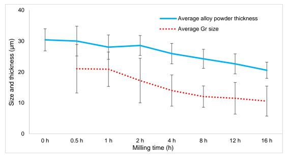
Figure 9. Average particle thickness of the as-received and milled composite powder.
