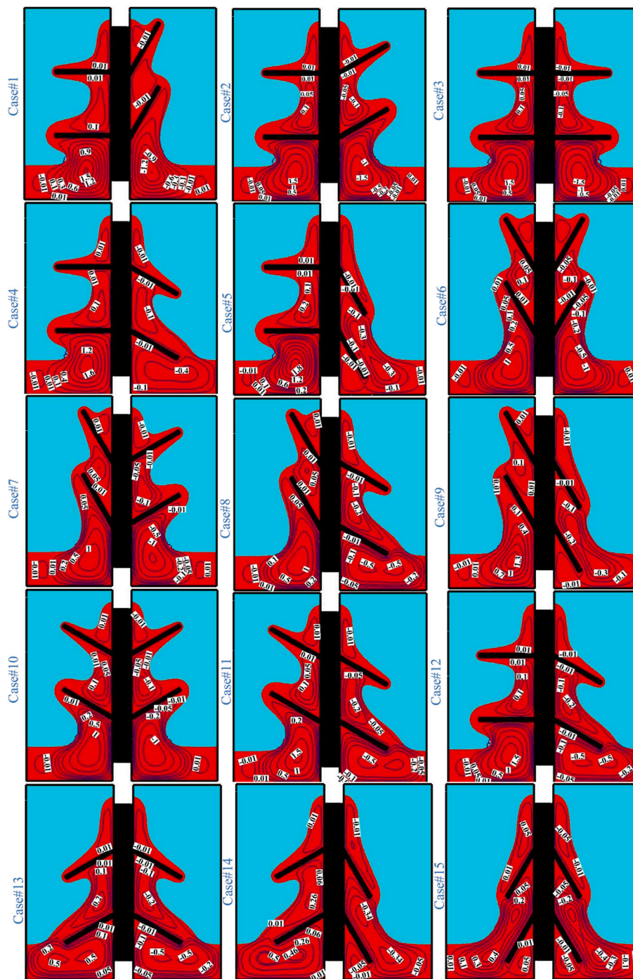
Fig. 7. Variation of streamlines in charged region (red color) respect to fin angle (non-symmetric cases) at Ste. = 0.09 , Ar = 8 , Ra = 1e5 (For interpretation of the references to color in this figure legend, the reader is referred to the web version of this article.)
