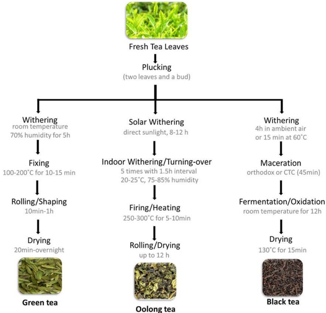
FIGURE 2.4 Tea production flow diagram. Adapted from Feng et al. (2019), Li et al. (2021b), Lin et al. (2016) and Theppakorn (2016).
