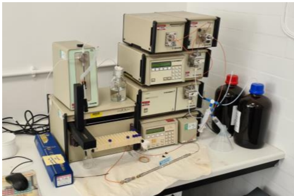
Fig 1: HPLC apparatus used to measure enantiomeric excess of pure products
