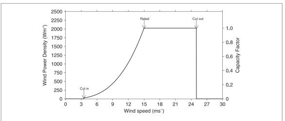
$\textbf{Figure 1.} \ I dealized wind-power transformation curve relating wind speed to power output and capacity factor (the fraction of maximum power produced). Units are $Wm^{-2}$ for power output.$
