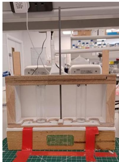
**Figure 2.1 – A photo of the rapid iterative negative geotaxis apparatus.**
