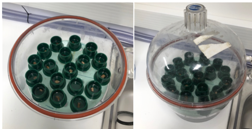
Figure 15. Human bone samples embedded in resin (left) and sealed in a desiccator vacuum (right). Source: author
