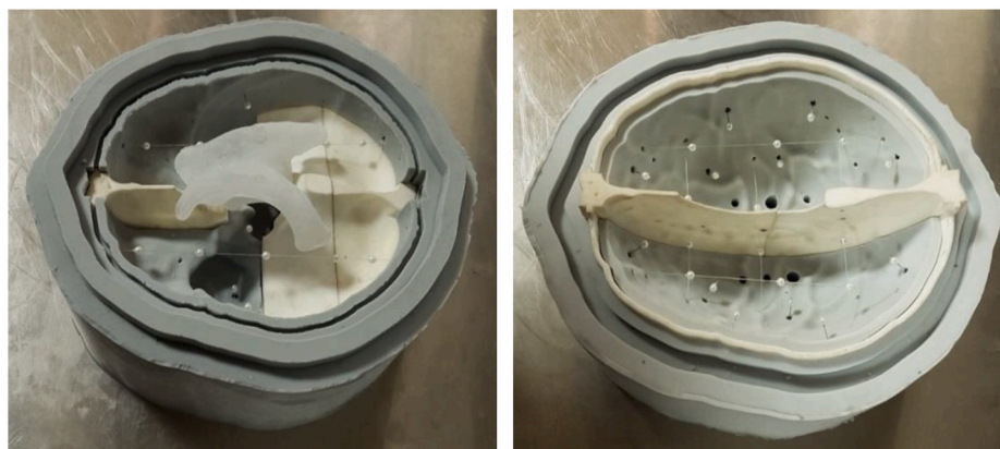
Fig. 2. Assembled lower (left) and upper (right) mould halves. Silicone mould components are grey in colour, rigid plastic inserts are off-white in colour and ice ventricle insert is the clouded structure in the middle of the left hand picture. Visible are also the brain shift imaging markers (glass beads) which are supported in the cavity with cantilevered map pins and gap-bridging fishing line (see Section 2.2.2).
