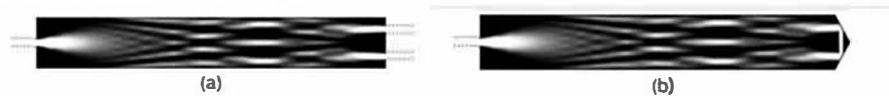
Figure 1: operation principle: (a) field distributions simulation of a 1 \times 2 MMI (b) the light reflectivity to the input waveguide due to positioning 45^\circ mirrors [1]
