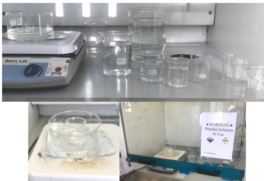
Figure 3.3: Top: Water bath placed on a hotplate at 95^\circ\text{C} , protected by a sheet of foil. Beakers containing water for the swirling rinse post etch; 600 ml, 150 ml, 100 ml. Two 100 ml beakers to receive the \text{H}_2\text{O}_2 and \text{H}_2\text{SO}_4 . Two 600 ml waste beakers used to hold tweezers and for any piranha solution waste. 1 L beaker filler with tap water that can be used to dilute waste or spills. Bottom left: Water bath at 95^\circ\text{C} with a 100 ml beaker containing 80 ml of piranha solution and eight Menzel Gläser 24x24 mm cover glasses held in place by a teflon coverslip holder (Fig. 3.1). Bottom right: Fume hood was closed and supervised during the etching process.
