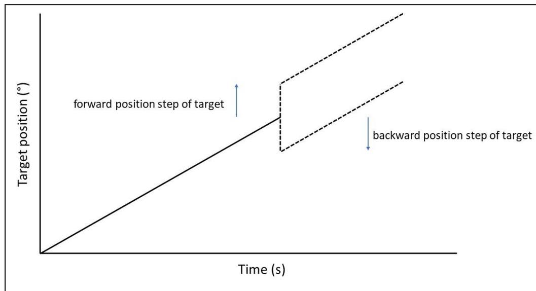
Figure 44 A schematic position time plot of a typical trial. The target (solid black line) travels with constant velocity until at some time it either steps forwards or backwards in position before continuing with constant velocity (dashed black line). The simulated step is used to evoke both catch up (step forward) and back up (step back) saccades. This paradigm will allow for exploring the properties of saccades made during smooth pursuit.
