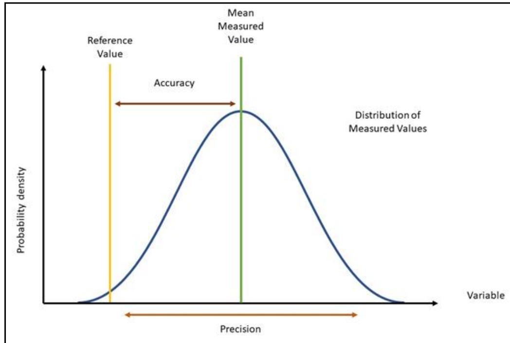
Figure 2: A one-dimensional schematic of the concepts of accuracy and precision. This diagram shows a hypothetical normal distribution (e.g. horizontal eye positions), the area under which sums to unity (i.e. 1). Accuracy represents the proximity of the mean measured value (e.g. the distance of the measured value from the reference value) while precision represents the spread of measured values).
