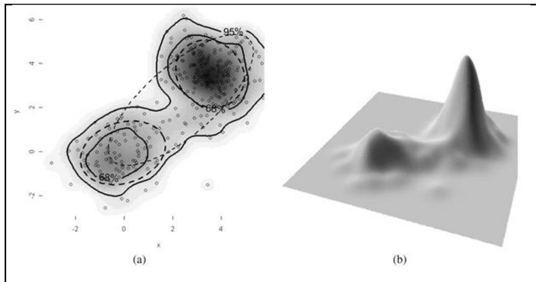
Figure 4 An example of both a BCEA and bPDF (Castet and Crossland 2012). The figure on the left shows a cluster of data points with two 'peaks'. A single BCEA (ellipse with 'thin' dashed line) has been fitted to that data. In addition, a bPDF has been fitted (contour with 'thick' dashed line). The bPDF considers that the underlying data is formed from two peaks (non-parametric), whereas the BCEA treats these data as being normally distributed along the x and y planes (parametric).
