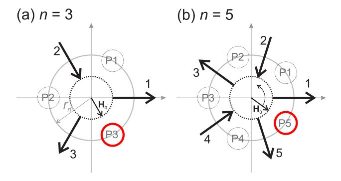
FIG. 1. (Color online) Radial odd-n spin ring systems for (a) n = 3, and (b) n = 5. The ring radius  $= r_n$ . Spins are number from i = 1 to n. An intrinsic ground state defect can take positions  $P_i$  as indicated by circles. The defect position for the given ground state configuration is emboldened in red at  $P_n$ .  $\mathbf{H}_0$  is the initial applied field used in simulations.
