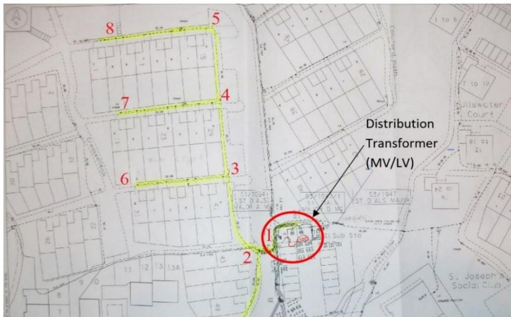
Figure C.1: Upper section of the low-voltage network showing the locations of Nodes N1 to N8.
