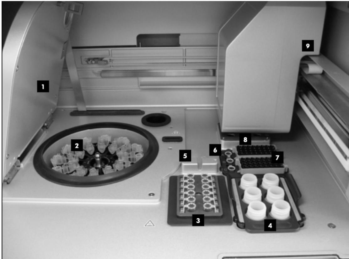
*Figure 7.3 Internal features of the QIAcube® machine. 1. Centrifuge lid; 2. Centrifuge; 3. Shaker; 4. Reagent bottle rack; 5. Tip sensor; 6. Microcentrifuge tube slots; 7. Tip racks; 8. Disposal slots for tips and columns; 9. Robotic arm. Source: QIAcube® User manual version 1.3 March 2018.*
