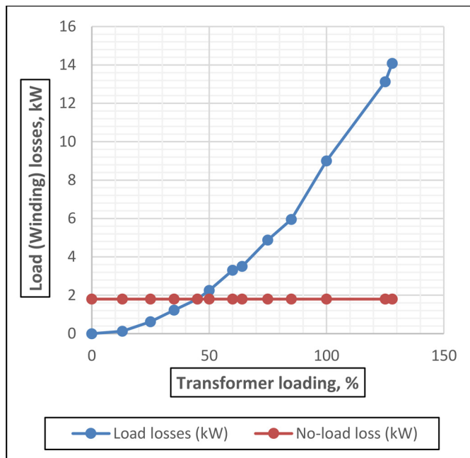
Fig. 9. Transformer Loading and load losses.
