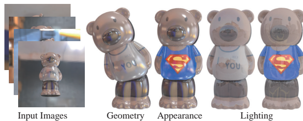
Figure 1: Given a set of input images, we train a neural radiance field that decouples geometry, appearance, and lighting. Our method supports not only the geometry manipulation and appearance editing but also the rendering of the captured or modified scene in a novel lighting condition.
