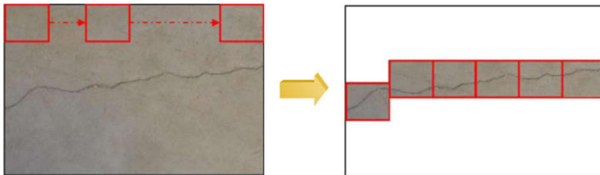
Figure 1: concrete crack detection by patch splitting and classification [7]
