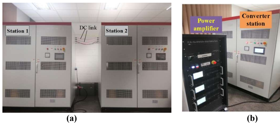
Figure 3.4. Laboratory scaled MVDC platform: (a) back-to-back cascaded 3L-NPC converter; (b) connection between the converter and a power amplifier.
