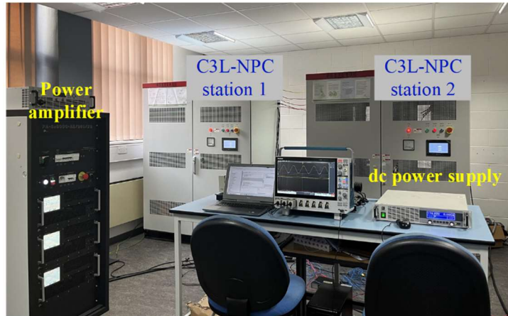
Figure 5.13. Three-terminal MVDC configuration consisting of two cascaded 3L-NPC converter stations and a DC power supply.
