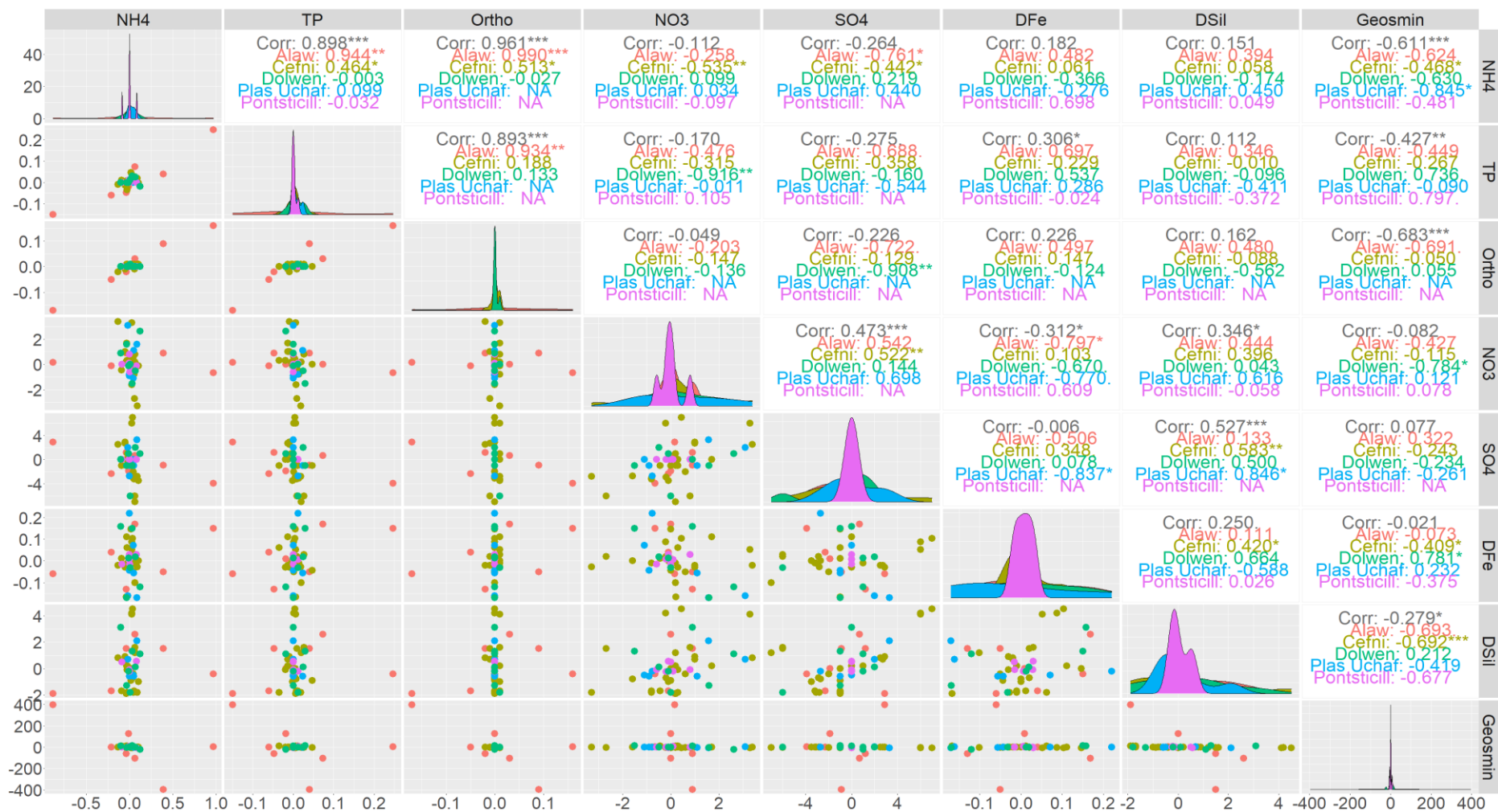
Figure 3.40: Correlogram of monthly changes in nutrients and monthly changes in geosmin concentrations for all reservoirs. Colour-coded by the individual reservoir. Pearson correlation is displayed on the right-hand side of the figure, and variable distribution is available on the diagonal. Correlation significance codes: ‘.’ p < 0.1 , p < 0.05 ‘*’, ‘**’ p < 0.01 , ‘***’ p < 0.001 .
