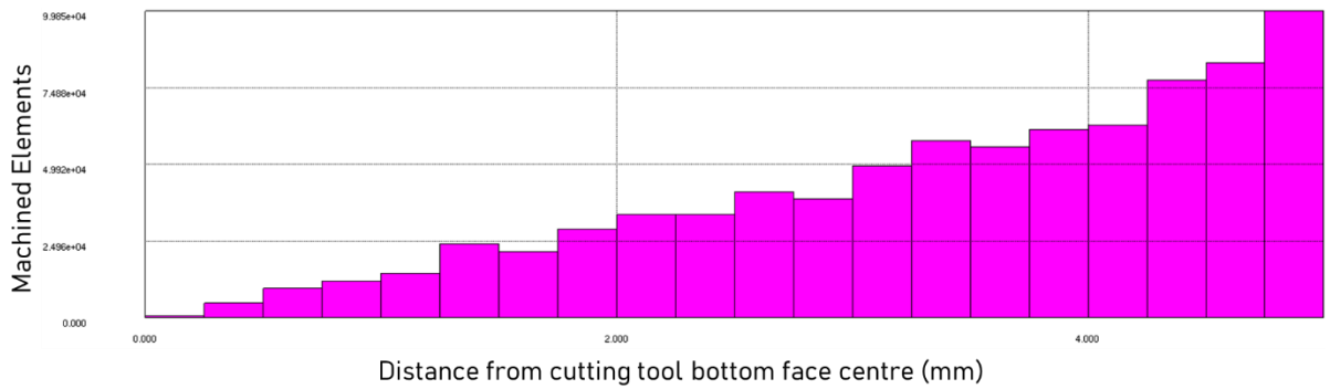
Figure 60 Radial cutting tool usage, simulation results.
