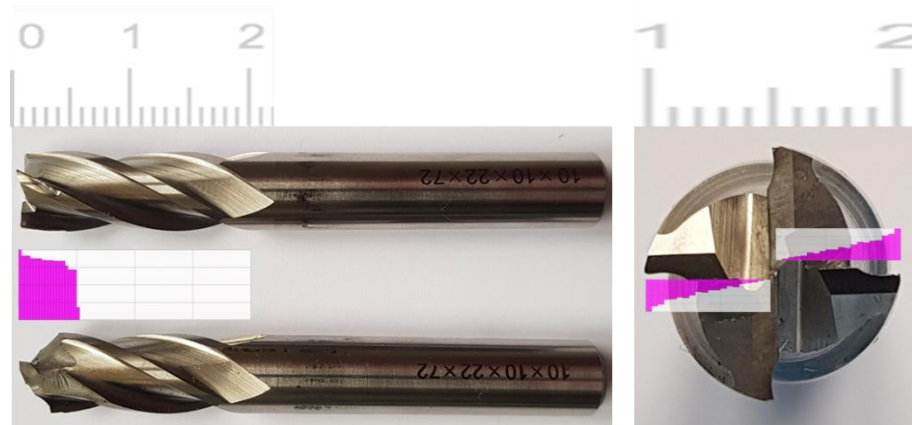
Figure 62 Cutting tools: Partially worn (top left and right) and catastrophically failed (bottom left).
