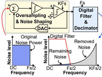
Fig. 10. Sigma-delta modulation.
