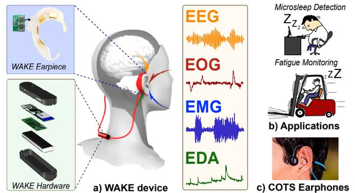
Fig. 1. Biosignals monitoring from behind the ears concept.
