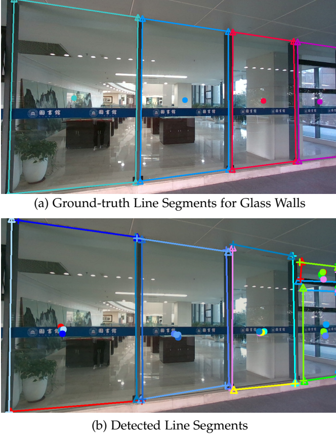
Fig. 10: An example of ground-truth and detected line segments: In the ground-truth (a), each glass instance is enclosed by at least three line segments, with its geometry center displayed as a circle matching the line segment color. Line segment endpoints are marked with triangles. For detected line segments (b), show the line segments with the top 22 classification scores, marking their endpoints with upward triangles and crosses. Each line segment has a predicted glass center, also shown as a circle.
