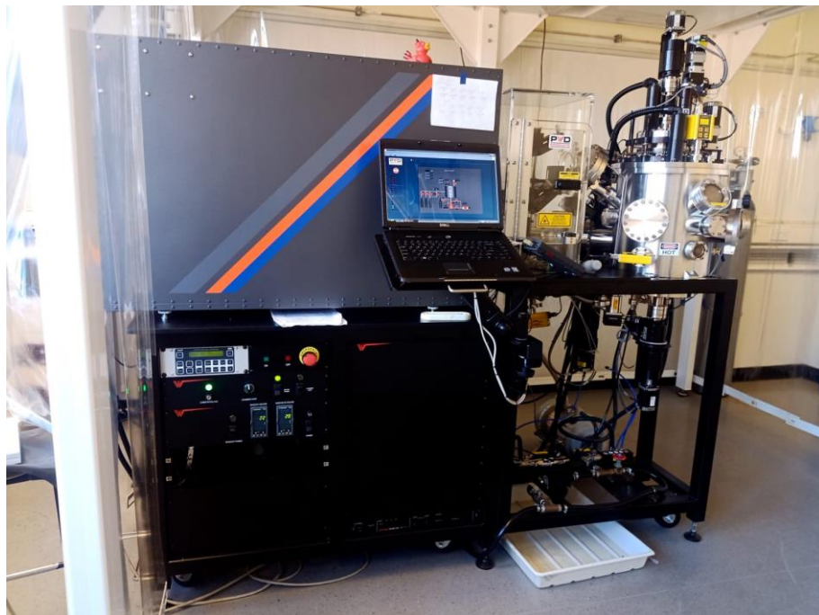
Figure 3.10: Pulsed Laser Deposition system with Titan magnetron sputtering subsystem.
